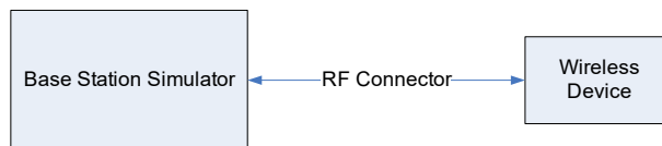
Figure 9-2 Power Measurement Setup
