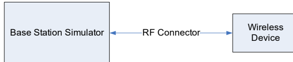
Figure 9-4 Power Measurement Setup
