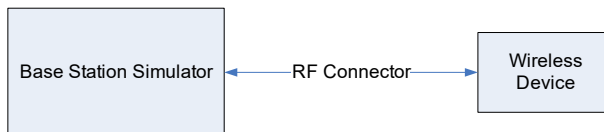
Figure 9-3 Power Measurement Setup
