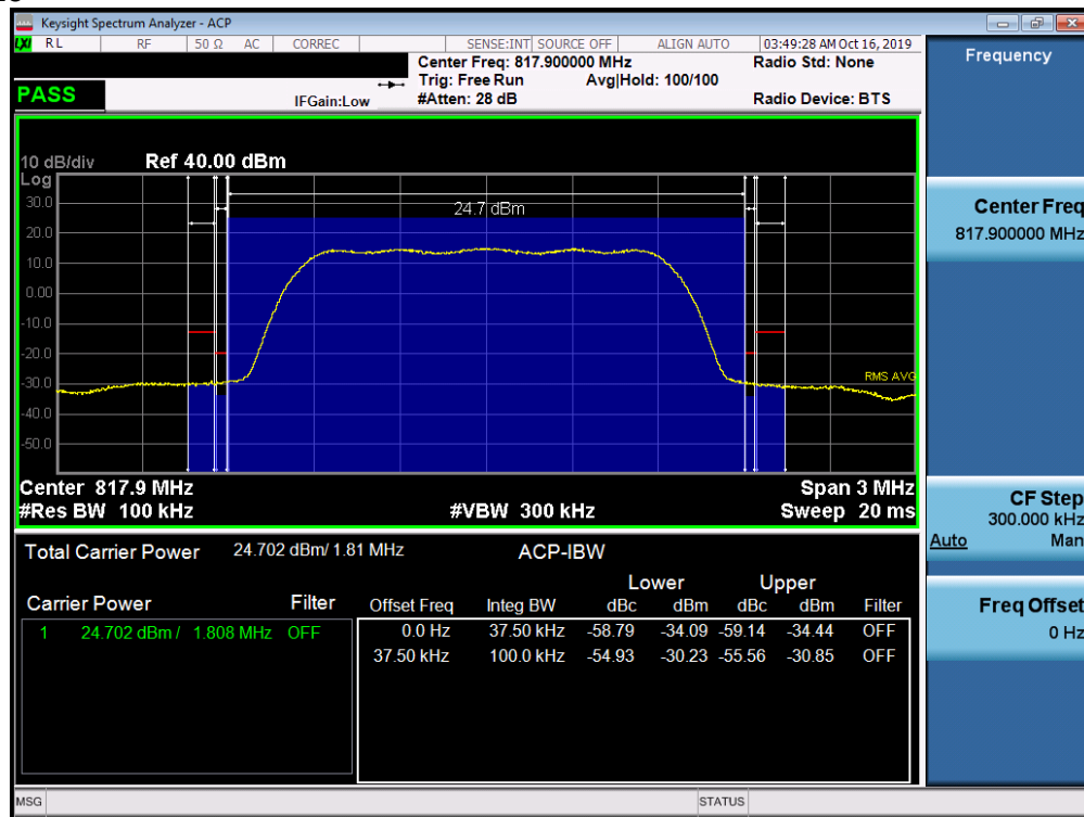
Plot 7-37. Channel Edge Plot (CDMA BC10 – Ch. 476)
