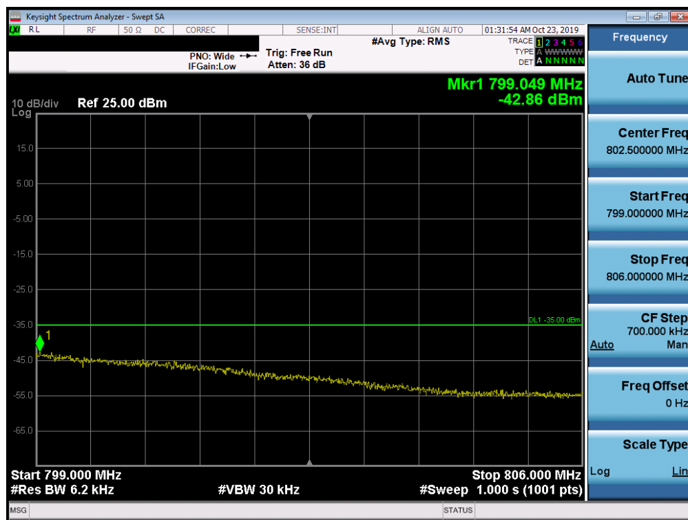
Plot 7-54. Upper Emission Mask Plot (LTE Band 14, 10MHz QPSK - RB Size 50)
