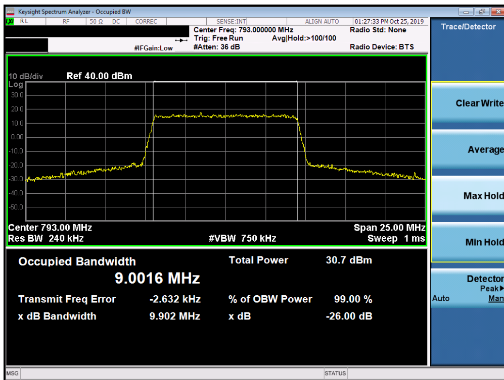
Plot 7-29. Occupied Bandwidth Plot (LTE Band 14 - 10MHz 64-QAM - Full RB Configuration)
