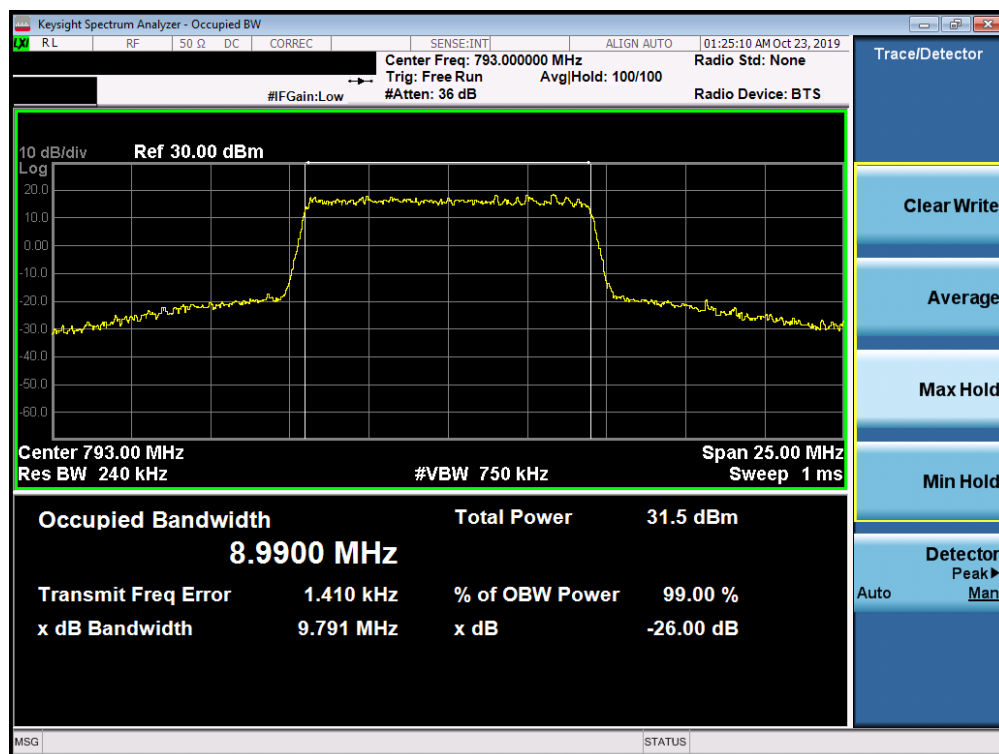
Plot 7-28. Occupied Bandwidth Plot (LTE Band 14 - 10MHz 16-QAM - Full RB Configuration)
