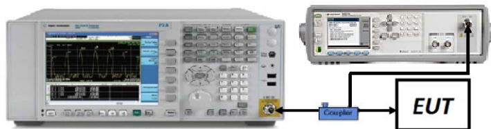
Figure 7-1. Test Instrument & Measurement Setup
