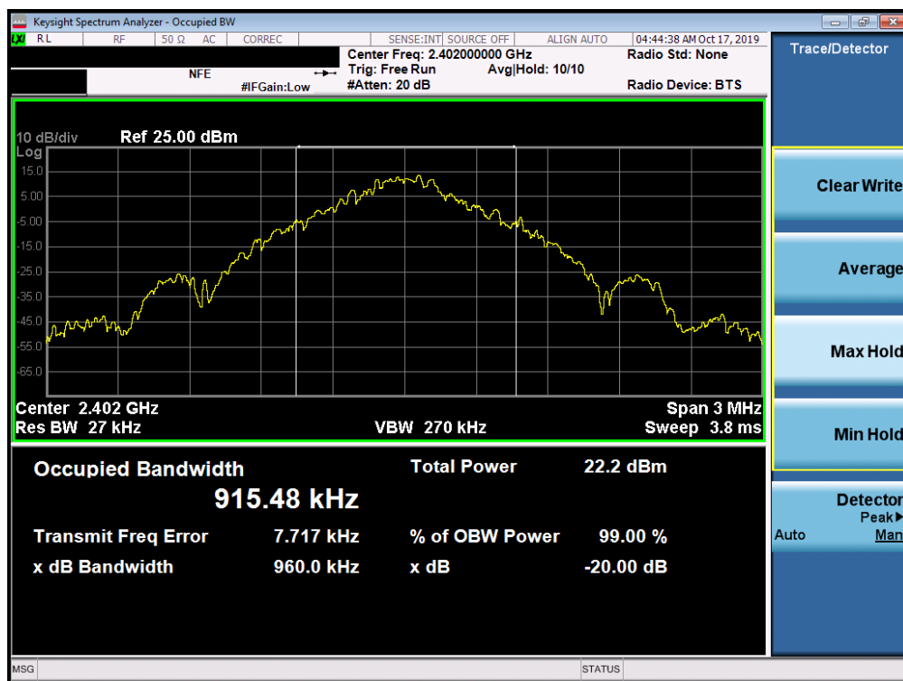
Plot 7-1. 20dB Bandwidth Plot (Bluetooth, 1Mbps – Ch. 0)
