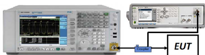
Figure 7-3. Test Instrument & Measurement Setup
