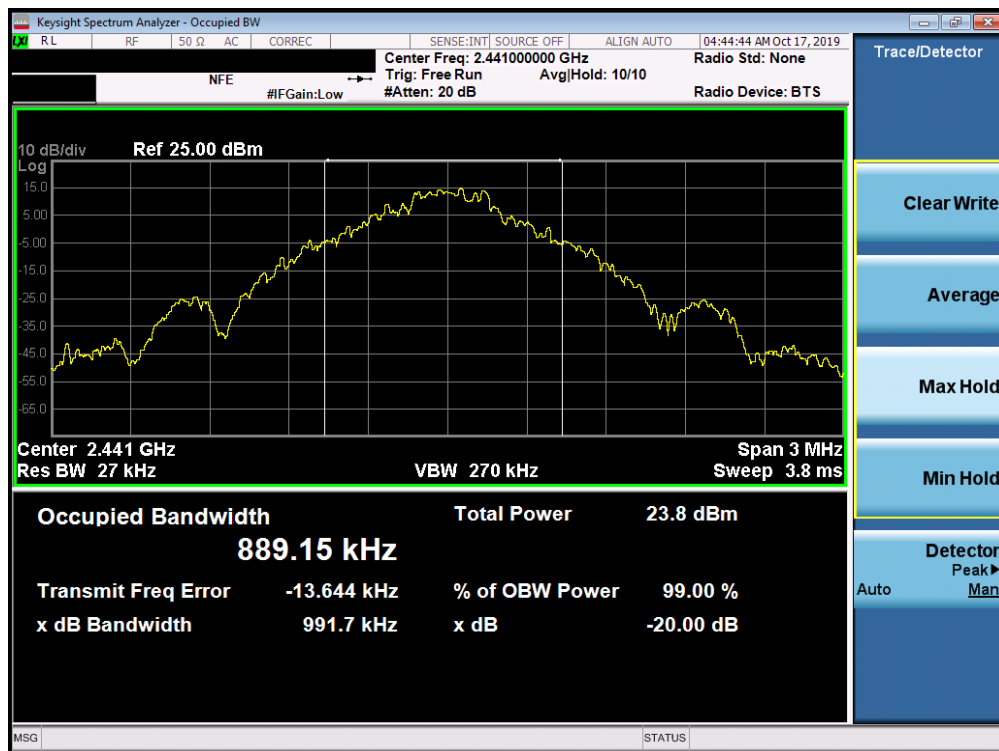
Plot 7-2. 20dB Bandwidth Plot (Bluetooth, 1Mbps – Ch. 39)
