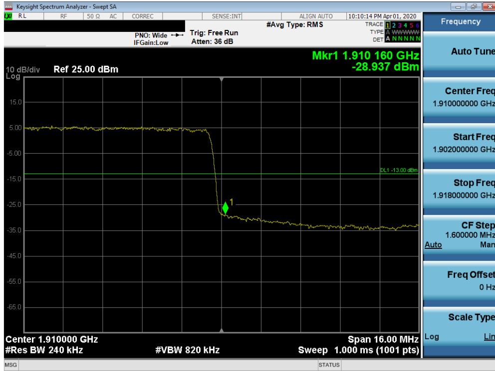
Plot 7-79. Upper Band Edge Plot (n2 - 20MHz DFT-s-OFDM-BPSK - Full RB Configuration)
