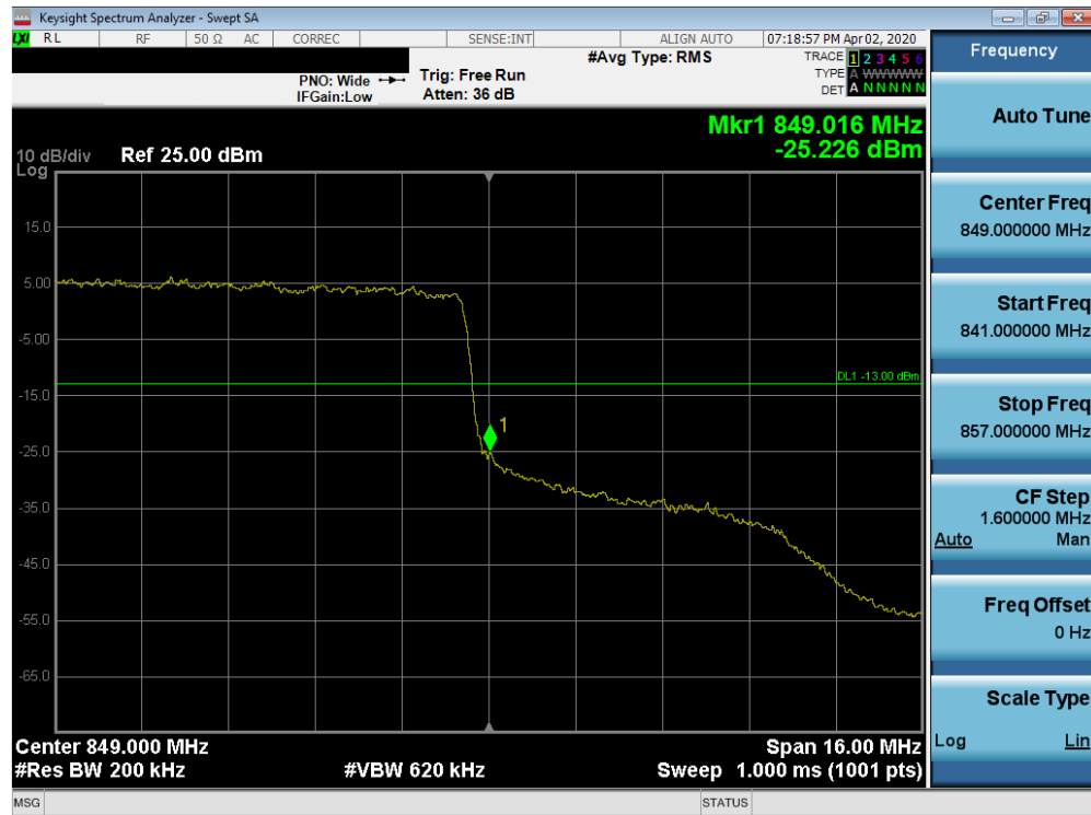
Plot 7-72. Upper Band Edge Plot (n5- 20MHz DFT-s-OFDM-BPSK - Full RB Configuration)
