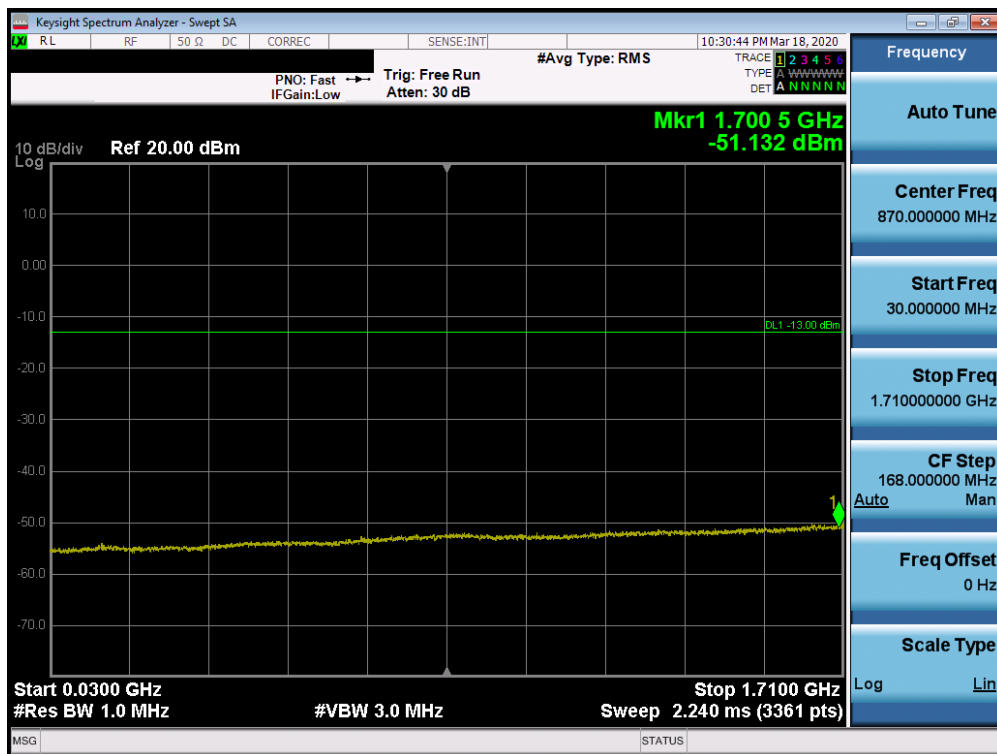
Plot 7-45. Conducted Spurious Plot (n66 - 20MHz DFT-s-OFDM-BPSK - RB Size 1, RB Offset 1 - Mid Channel)
