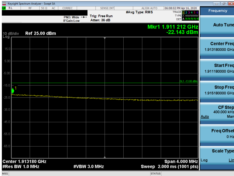
Plot 7-80. Upper Extended Band Edge Plot (n2 - 20MHz DFT-s-OFDM-BPSK - Full RB Configuration)
