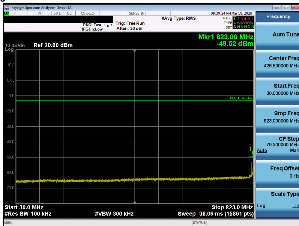
Plot 7-33. Conducted Spurious Plot (n5 - 20MHz DFT-s-OFDM -BPSK - RB Size 1, RB Offset 1 – Low Channel)
