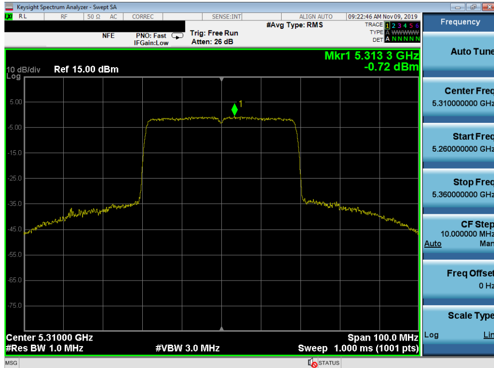
Plot 7-92. Power Spectral Density Plot SISO ANT1 (40MHz BW 802.11ax – Full Tones (UNII Band 2A) – Ch. 62)
