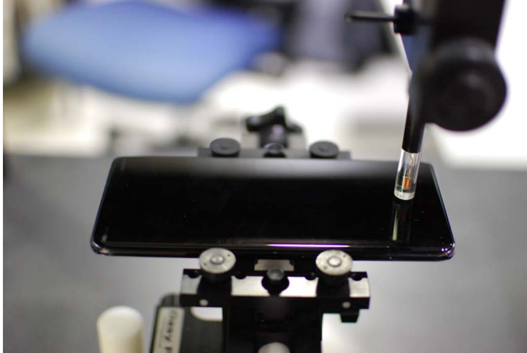
Figure 13-1 Test Setup for Wireless Device
