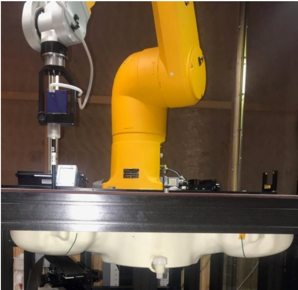
Figure 7-1 SAR measurement setup
