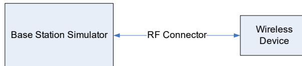
Figure 9-1 Power Measurement Setup
