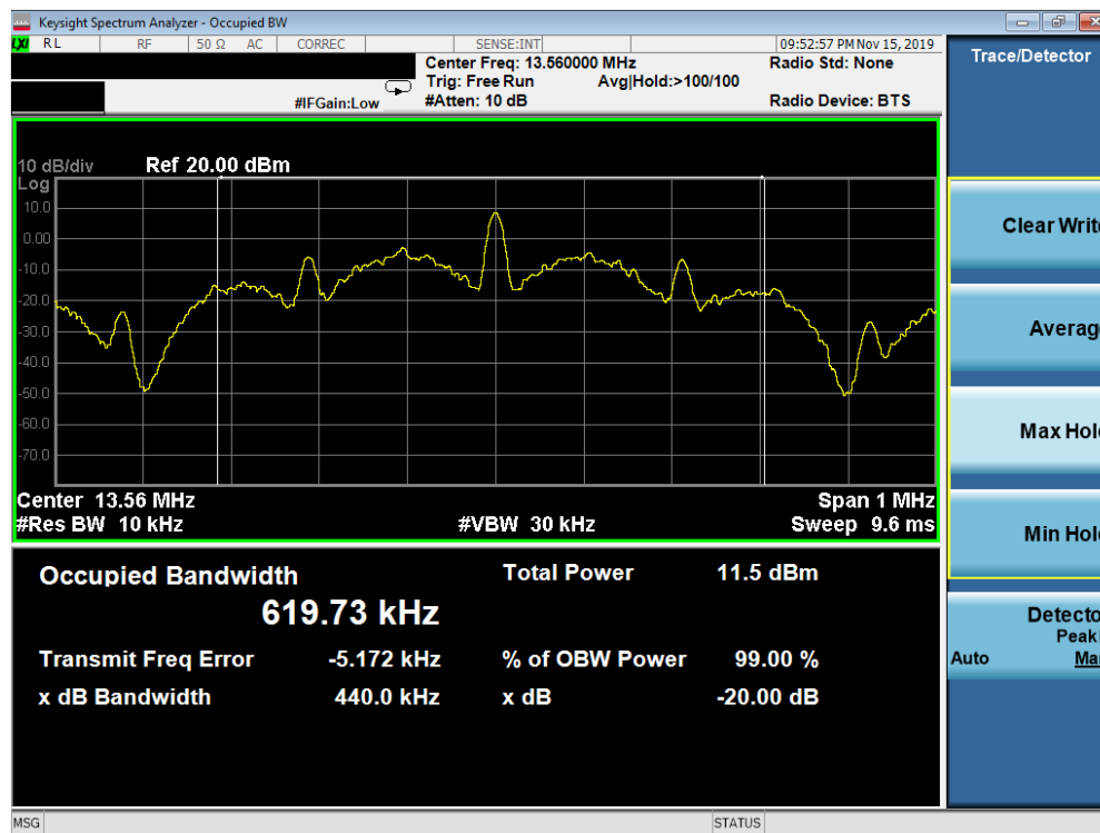
Figure 7-2. Occupied Bandwidth Plot
