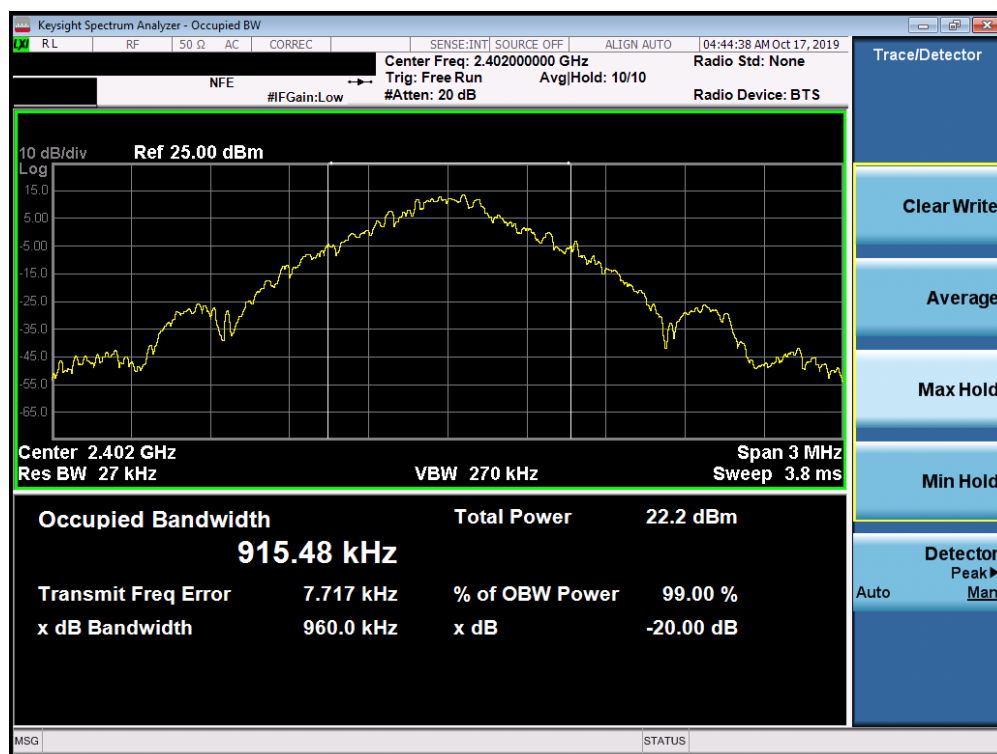
Plot 7-1. 20dB Bandwidth Plot (Bluetooth, 1Mbps – Ch. 0)
