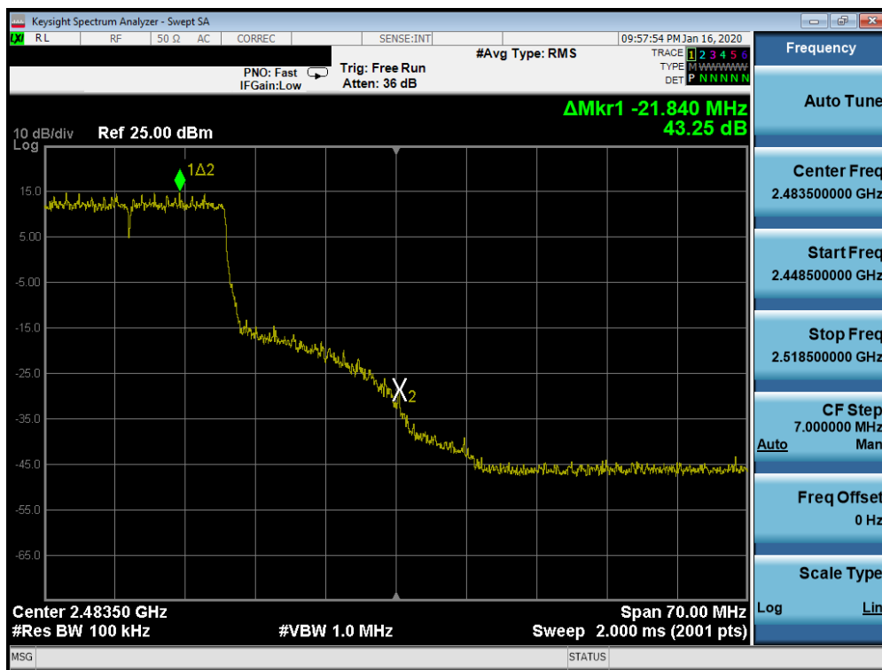
Plot 7-45. Band Edge Plot SISO ANT2 (802.11ax OFDMA – 242 Tones – Ch. 10)
