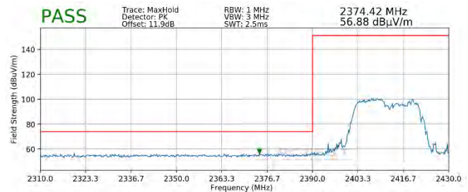
Plot 7-105. Radiated Restricted Lower Band Edge Measurement SISO ANT2 (Peak – 106 Tones)
