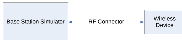
Figure 9-3 Power Measurement Setup
