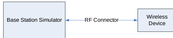
Figure 9-1 Power Measurement Setup
