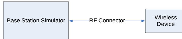
Figure 9-4 Power Measurement Setup
