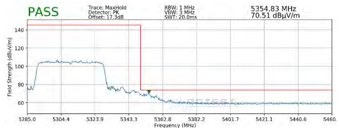
Plot 7-359. Radiated Upper Band Edge Plot MIMO (Peak – UNII Band 2A – 484 Tones)
