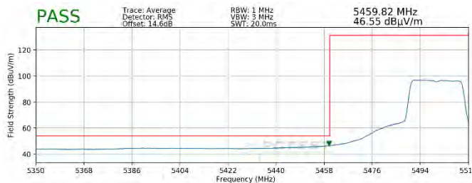
Plot 7-353. Radiated Lower Band Edge Plot MIMO (Average - UNII Band 2C - 242 Tones)
