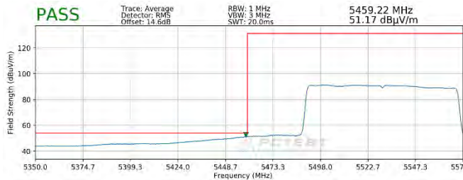
Plot 7-346. Radiated Lower Band Edge Plot SISO ANT2 (Average - UNII Band 2C - 996 Tones)
