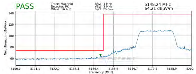
Plot 7-350. Radiated Lower Band Edge Plot MIMO (Peak - UNII Band 1 - 242 Tones)
