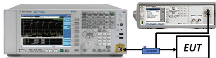
Figure 7-3. Test Instrument & Measurement Setup
