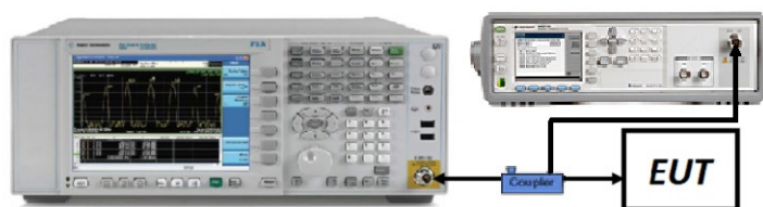
Figure 7-1. Test Instrument & Measurement Setup
