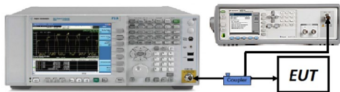
Figure 7-6. Test Instrument & Measurement Setup
