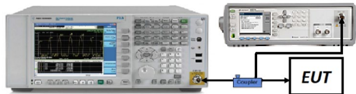
Figure 7-2. Test Instrument & Measurement Setup
