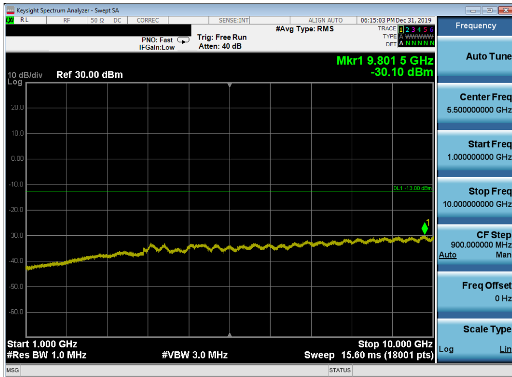
Plot 7-621. Conducted Spurious Plot (n5 - 20MHz DFT-s-OFDM-QPSK - RB Size 1, RB Offset 1 - Mid Channel)
