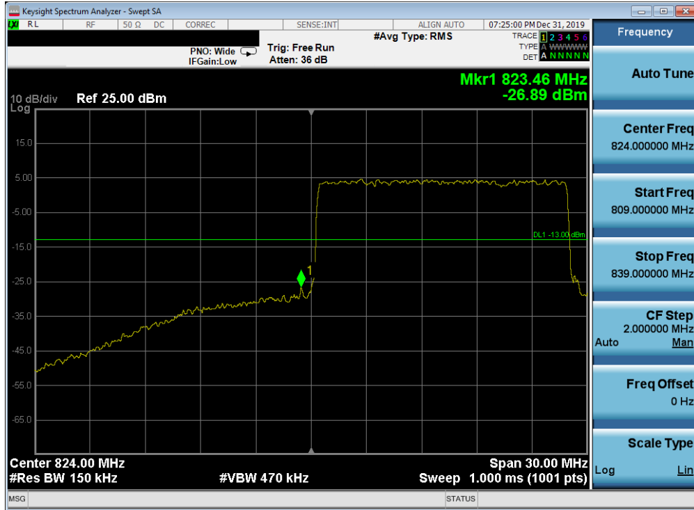
Plot 7-664. Lower Band Edge Plot (n5 - 15MHz DFT-s-OFDM-QPSK - Full RB Configuration)
