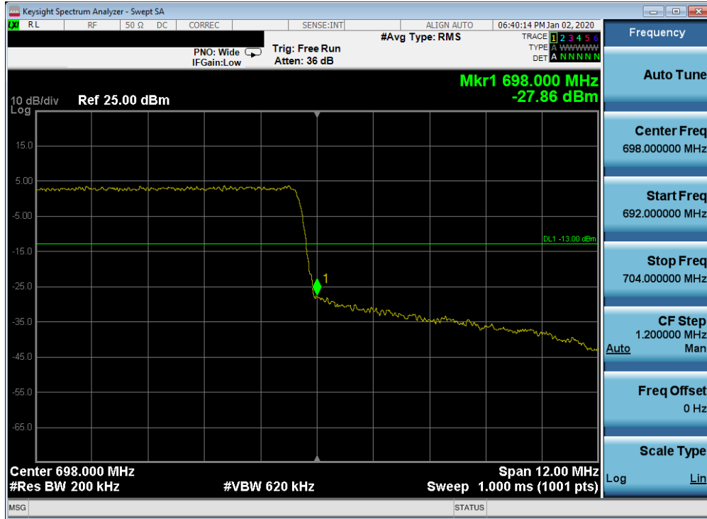
Plot 7-657. Upper Band Edge Plot (n71 - 15MHz CP-OFDM-QPSK - Full RB Configuration)
