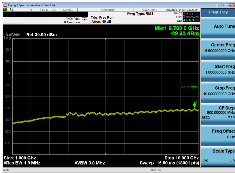
Plot 7-615. Conducted Spurious Plot (n71 - 20MHz DFT-s-OFDM-QPSK - RB Size 1, RB Offset 1 - High Channel)
