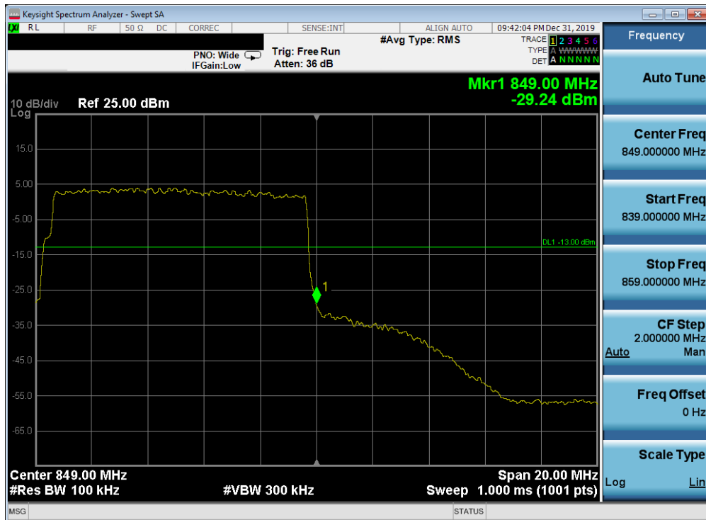
Plot 7-663. Upper Band Edge Plot (n5 - 10MHz DFT-s-OFDM-QPSK - Full RB Configuration)
