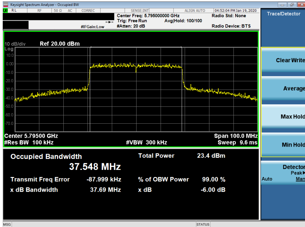
Plot 7-130. 6dB Bandwidth Plot SISO ANT2 (40MHz BW 802.11ax (UNII Band 3) – Ch. 159)
