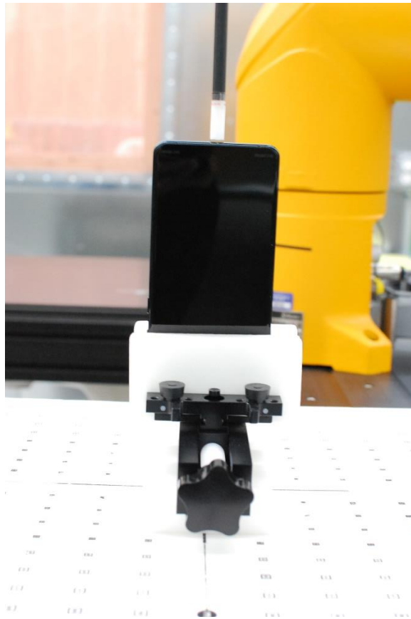
Near-Field Power Density Test Setup Photo 4 – Top Edge at 2 mm
