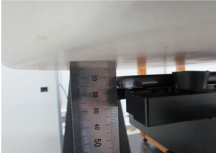
Distance of 10 mm from the EUT
