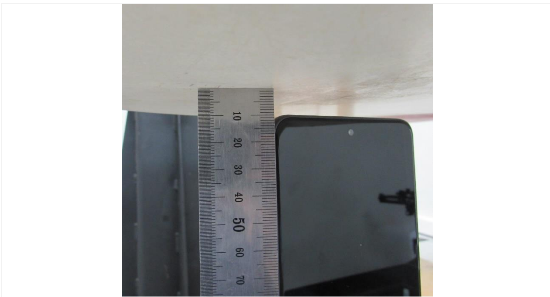
Distance of 10 mm from the EUT
