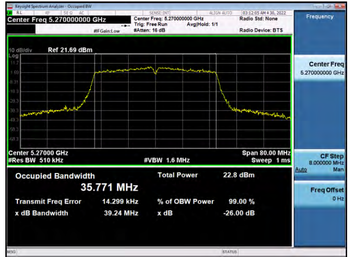
802.11n_HT40 UNII 3 BAND 26 dB Bandwidth (CH 159)
