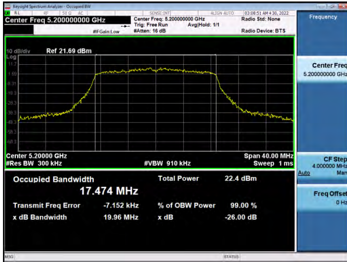
802.11ac_VHT20 UNII 2C BAND 26 dB Bandwidth(CH 144)
