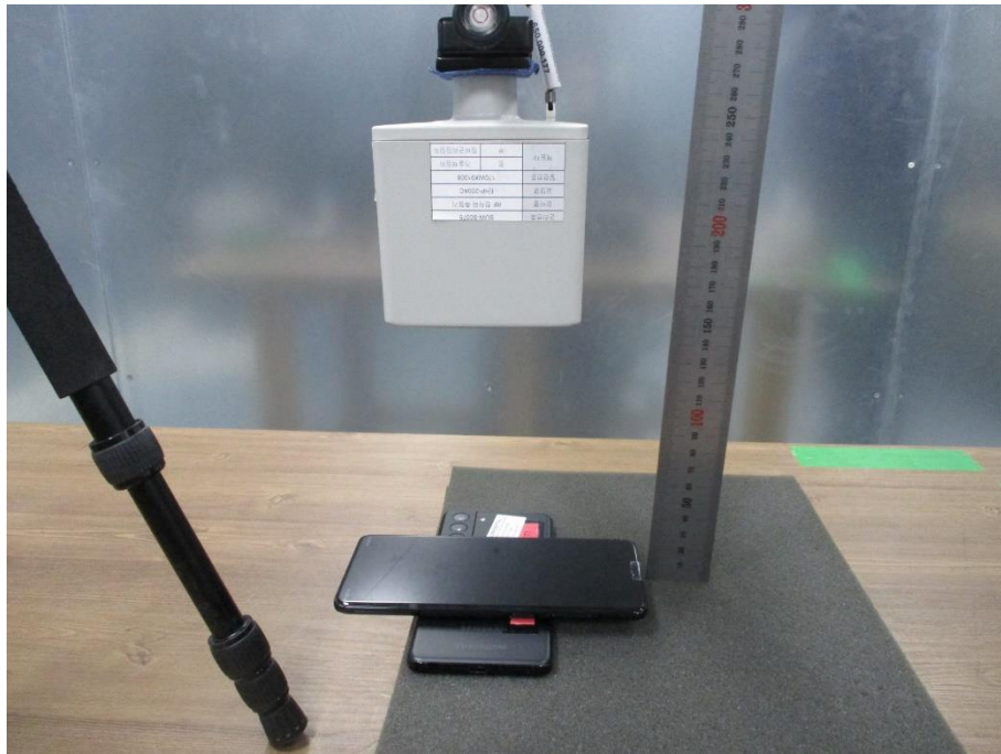
Top charger below client (20cm distance)
