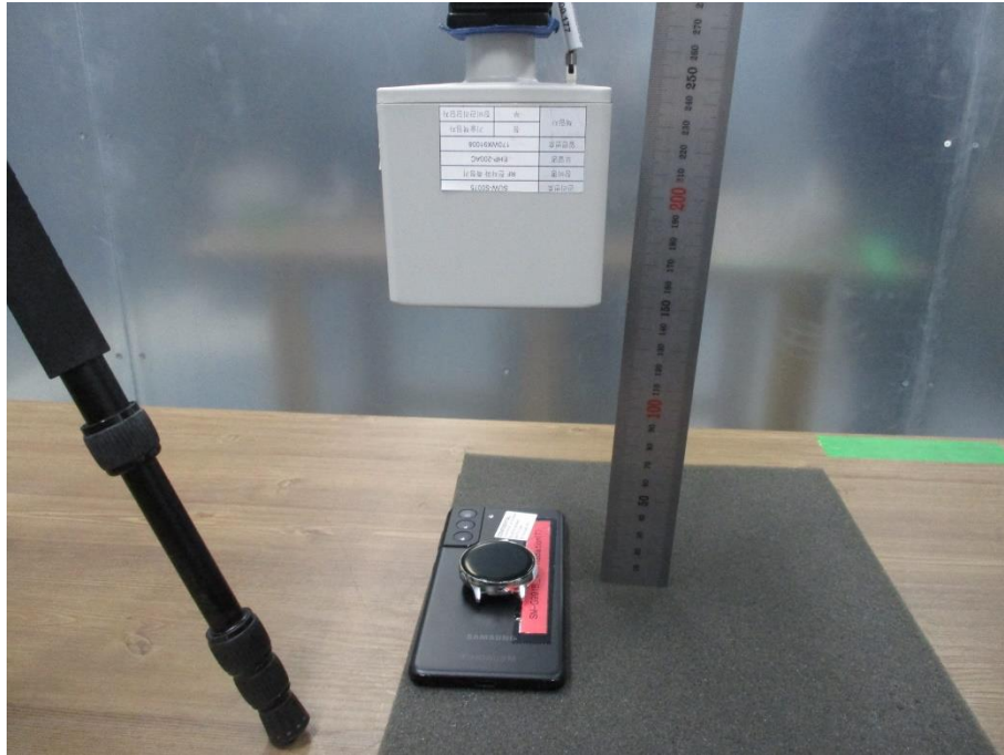
Top charger below client (20cm distance)
