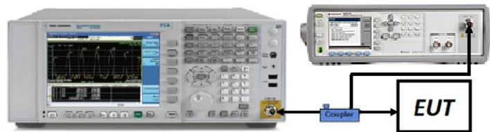
Figure 7-6. Test Instrument & Measurement Setup
