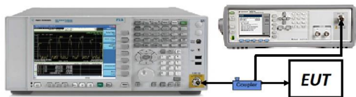
Figure 7-5. Test Instrument & Measurement Setup
