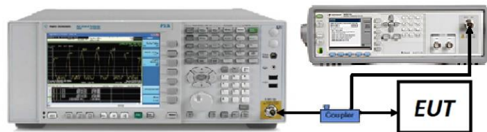
Figure 7-1. Test Instrument & Measurement Setup
