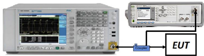
Figure 7-4. Test Instrument & Measurement Setup
