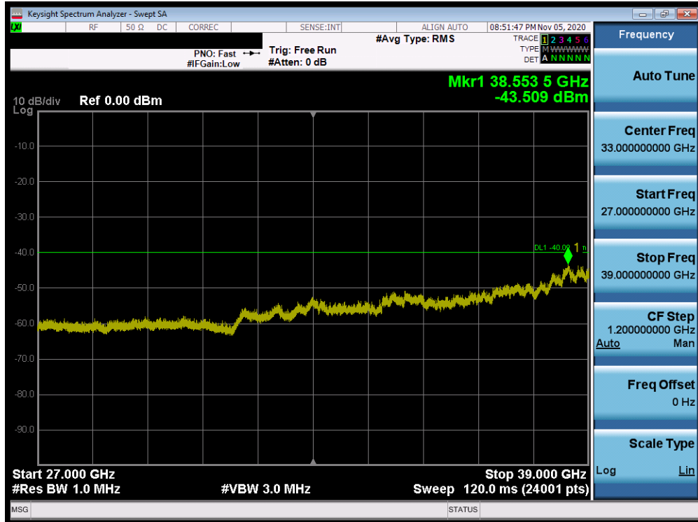
Plot 7-56. Conducted Spurious Plot (Band 48 – 20.0MHz QPSK – PCC 1/99 SCC 1/0 – Low Channel)
