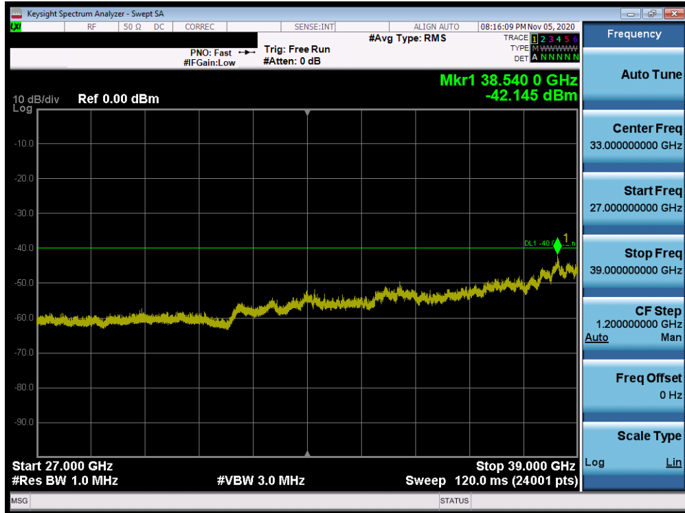
Plot 7-64. Conducted Spurious Plot (Band 48 – 20.0MHz QPSK – PCC 1/0 SCC 1/99 – High Channel)
