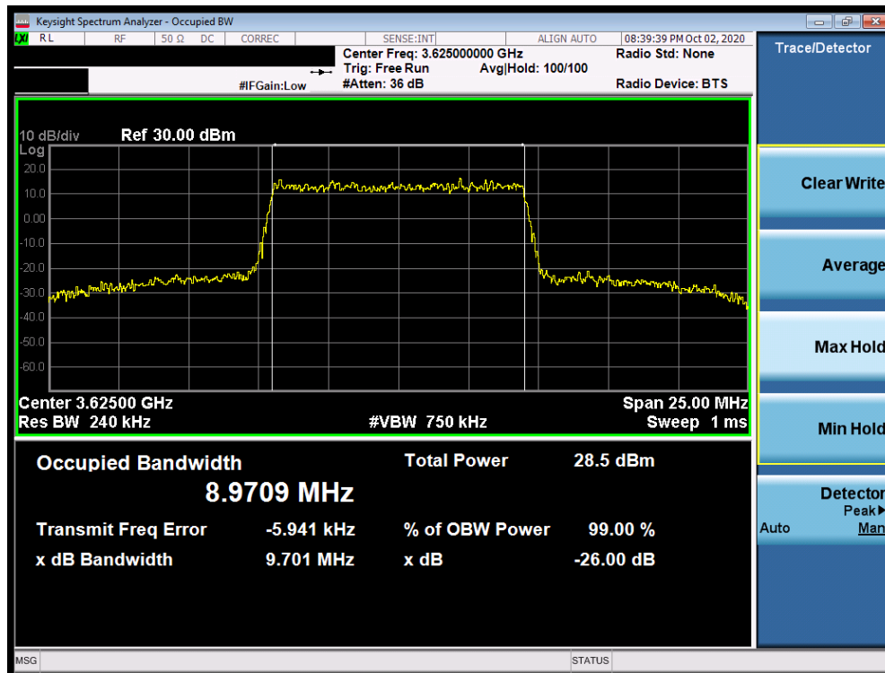
Plot 7-10. Occupied Bandwidth Plot (LTE Band 48 - 10.0MHz 16-QAM - Full RB Configuration)
