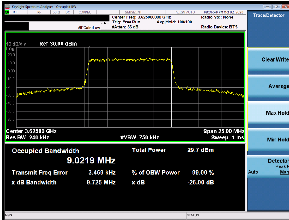
Plot 7-9. Occupied Bandwidth Plot (LTE Band 48 - 10.0MHz QPSK - Full RB Configuration)
