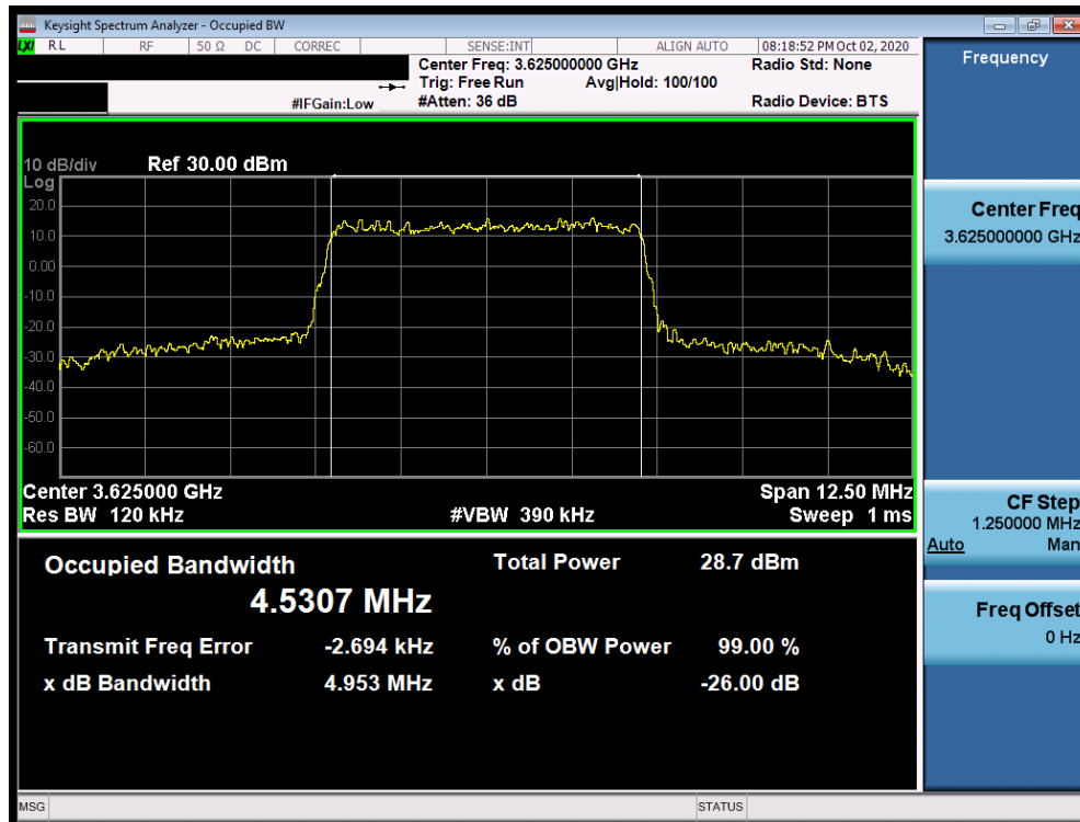
Plot 7-14. Occupied Bandwidth Plot (LTE Band 48 - 5.0MHz 16-QAM - Full RB Configuration)
