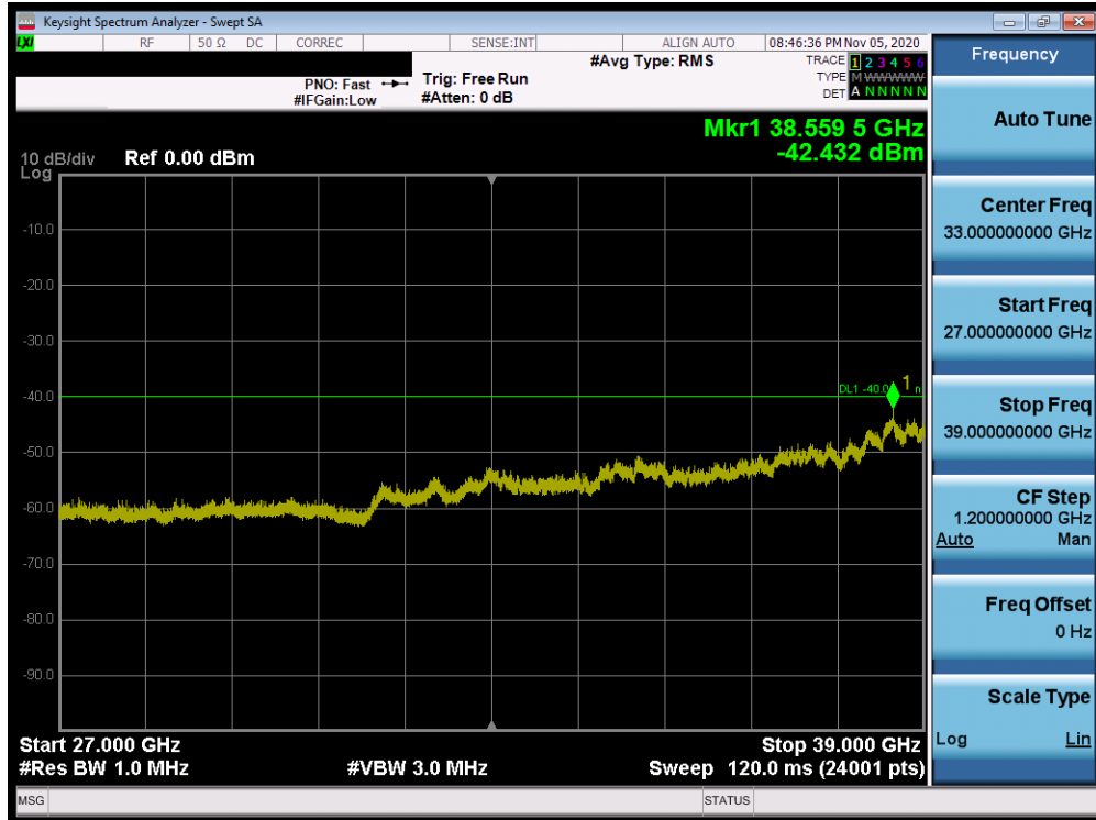
Plot 7-60. Conducted Spurious Plot (Band 48 – 20.0MHz QPSK – PCC 1/99 SCC 1/0 – Mid Channel)
