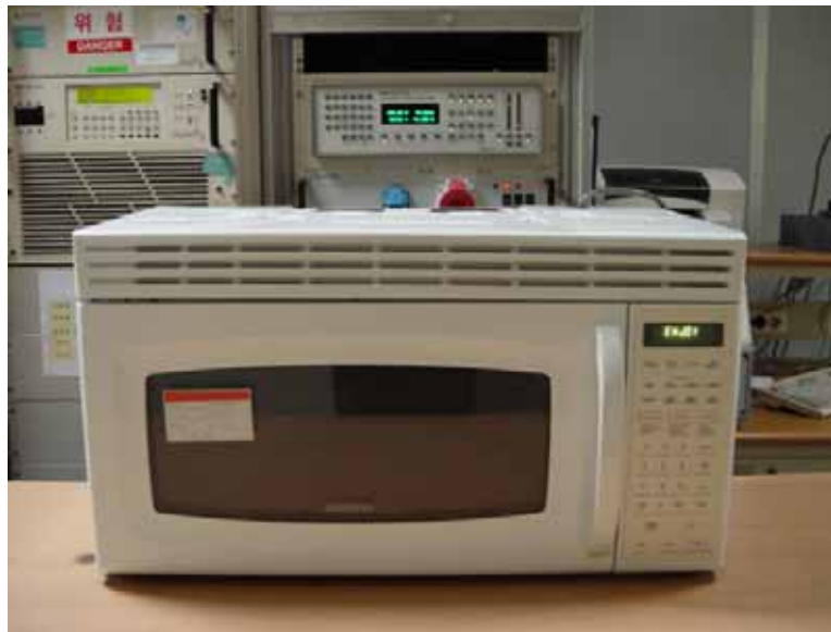
Fig.3 Test Setup for RF output power
