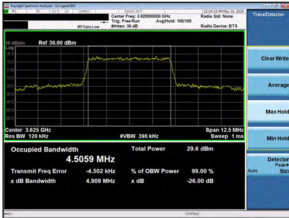
Plot 7-3. Occupied Bandwidth Plot (Band 48 - 5.0MHz 64-QAM - Full RB Configuration)
