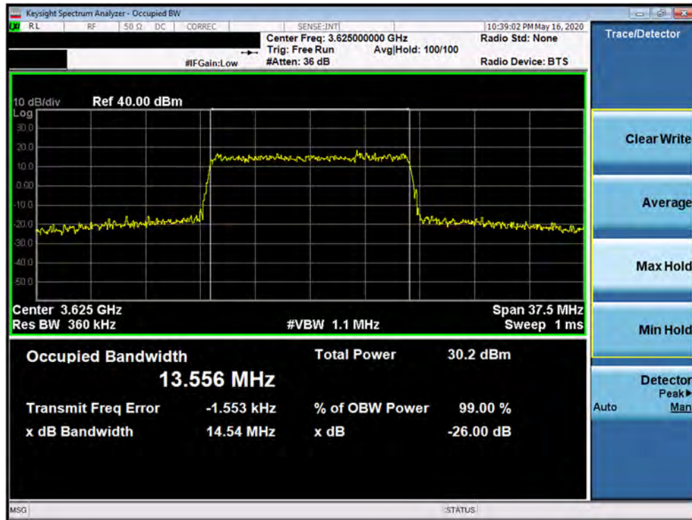
Plot 7-9. Occupied Bandwidth Plot (Band 48 - 15.0MHz 64-QAM - Full RB Configuration)
