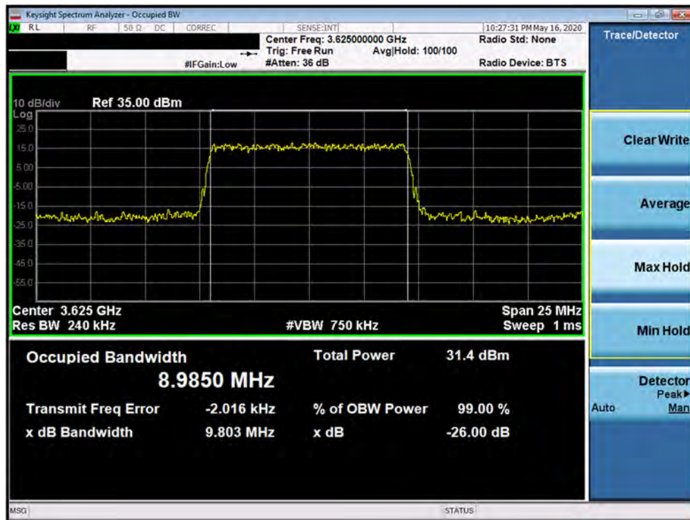
Plot 7-4. Occupied Bandwidth Plot (Band 48 - 10.0MHz QPSK - Full RB Configuration)
