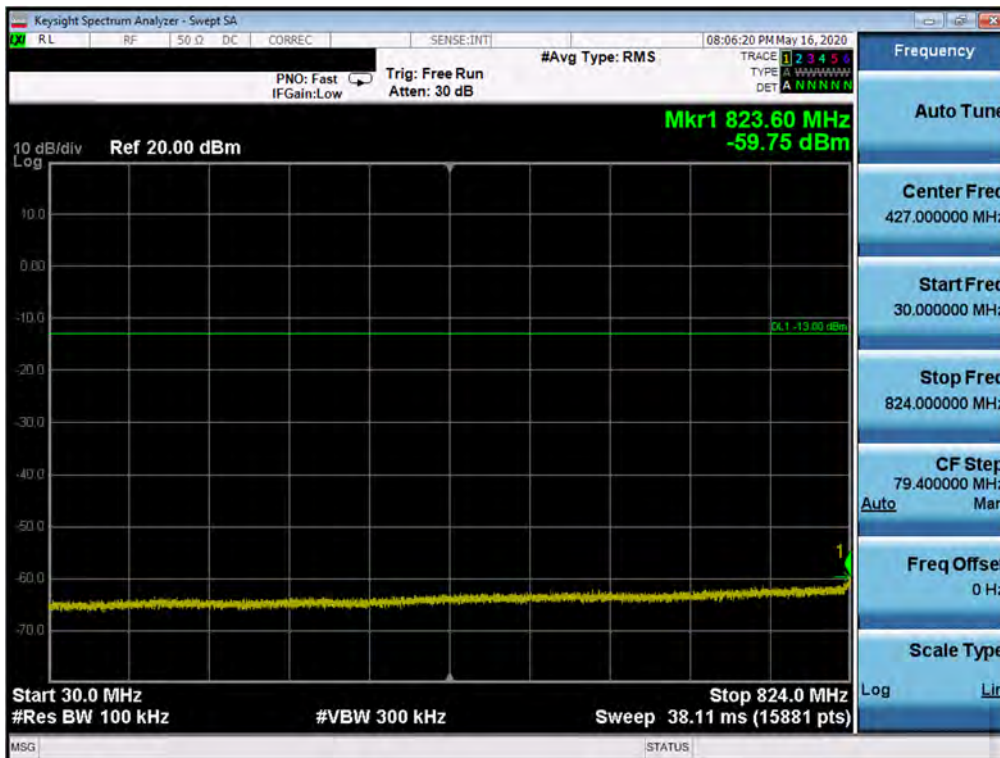
Plot 7-369. Conducted Spurious Plot (Band 5 – 10 + 10 MHz QPSK – PCC 1/49 SCC 1/0 – High Channel)
