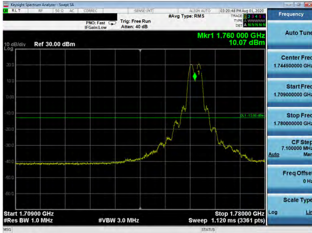
Plot 7-383. Conducted Spurious Plot (Band 66 – 20 + 20 MHz QPSK – PCC 1/99 SCC 1/0 – High Channel)
