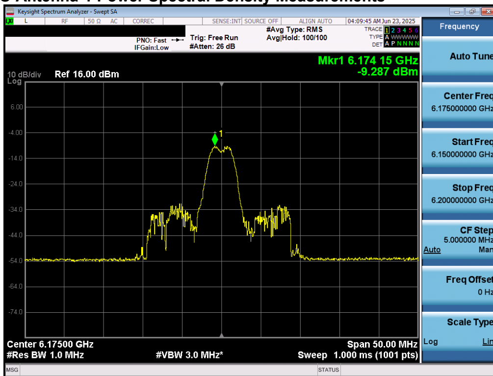
Plot 7-29. Power Spectral Density Plot MIMO ANT1 (20MHz 802.11ax/be (26 Tones) (UNII Band 5) – Ch. 45) - VLP
