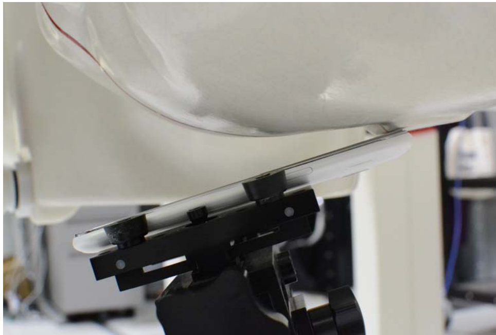
SAR Test Setup Photo 4: Left Tilt
