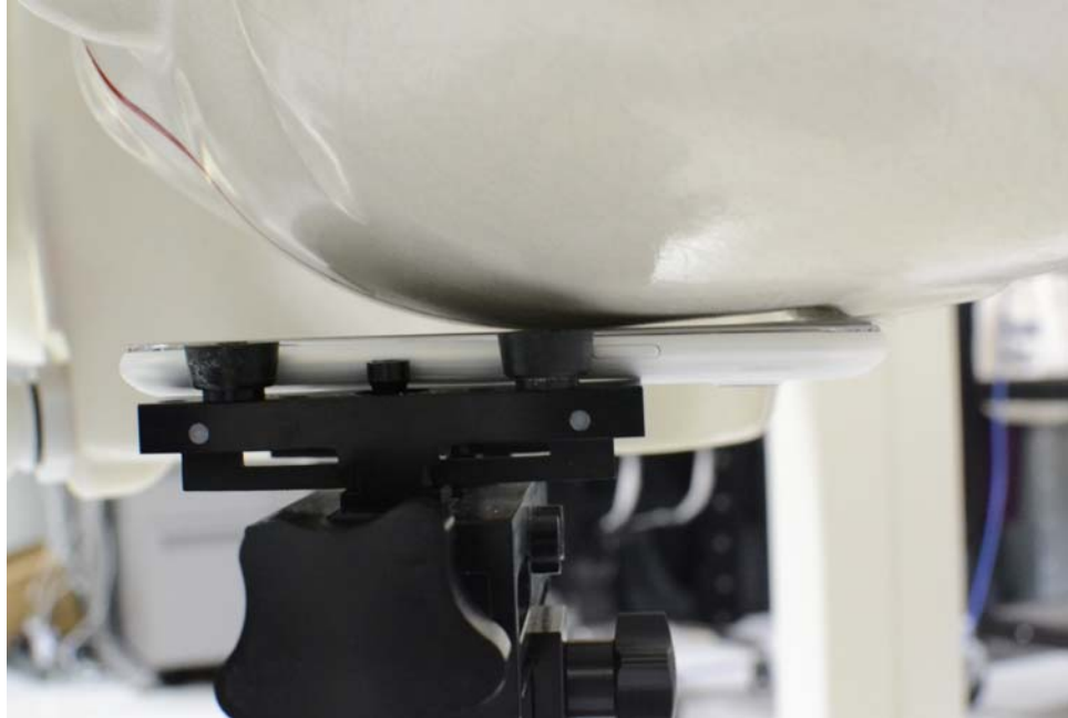
SAR Test Setup Photo 3: Left Cheek
