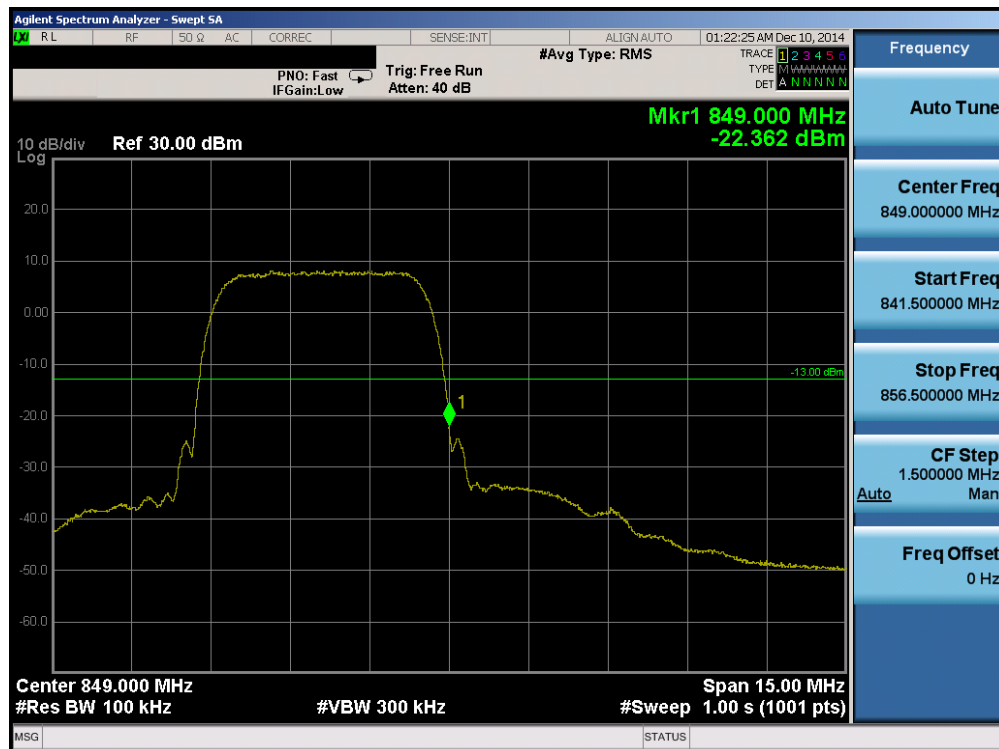
Plot 6-32. Band Edge Plot (Cellular WCDMA Mode – Ch. 4233)
