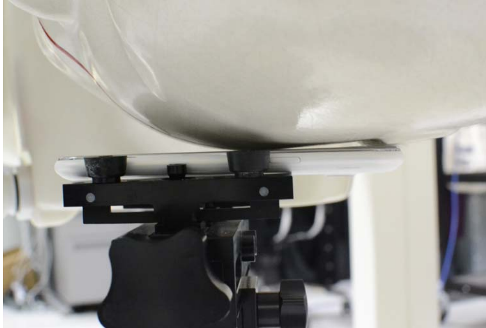
SAR Test Setup Photo 3: Left Cheek
