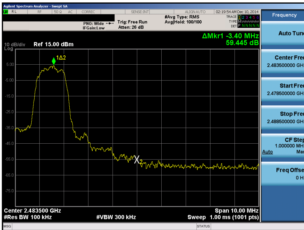
Plot 6-29. Band Edge Plot (Bluetooth with Hopping Disabled, 3 Mbps – Ch. 78)
