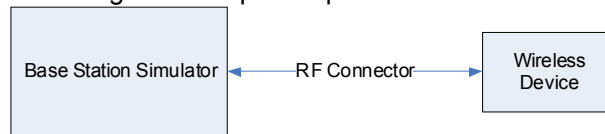
Figure 9-2 Power Measurement Setup
