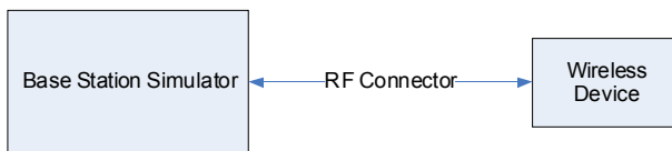
Figure 9-1 Power Measurement Setup
