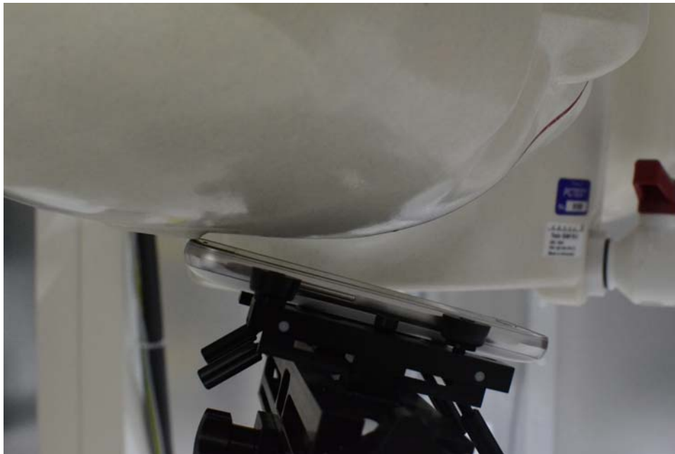
SAR Test Setup Photo 2: Right Tilt
