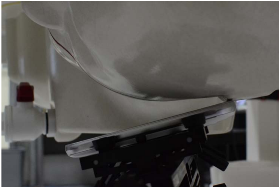
SAR Test Setup Photo 4: Left Tilt
