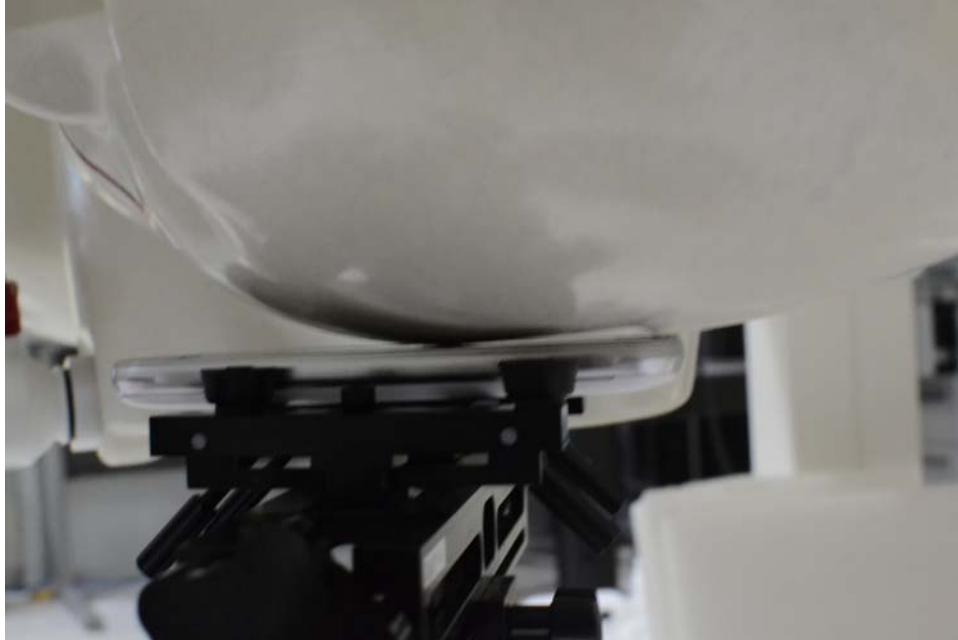
SAR Test Setup Photo 3: Left Cheek
