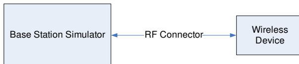
Figure 9-1 Power Measurement Setup
