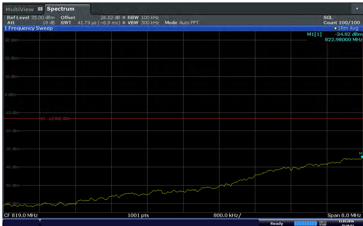
Plot 6-30. Extended Lower Band Edge Plot (Band 5 – 5.0MHz – 16QAM – RB Size 25)
