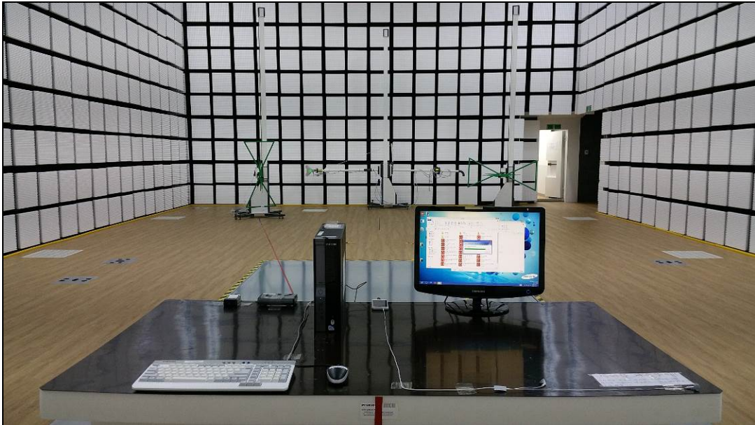
[ Radiated Disturbance for Below 1 GHz – Front ]
