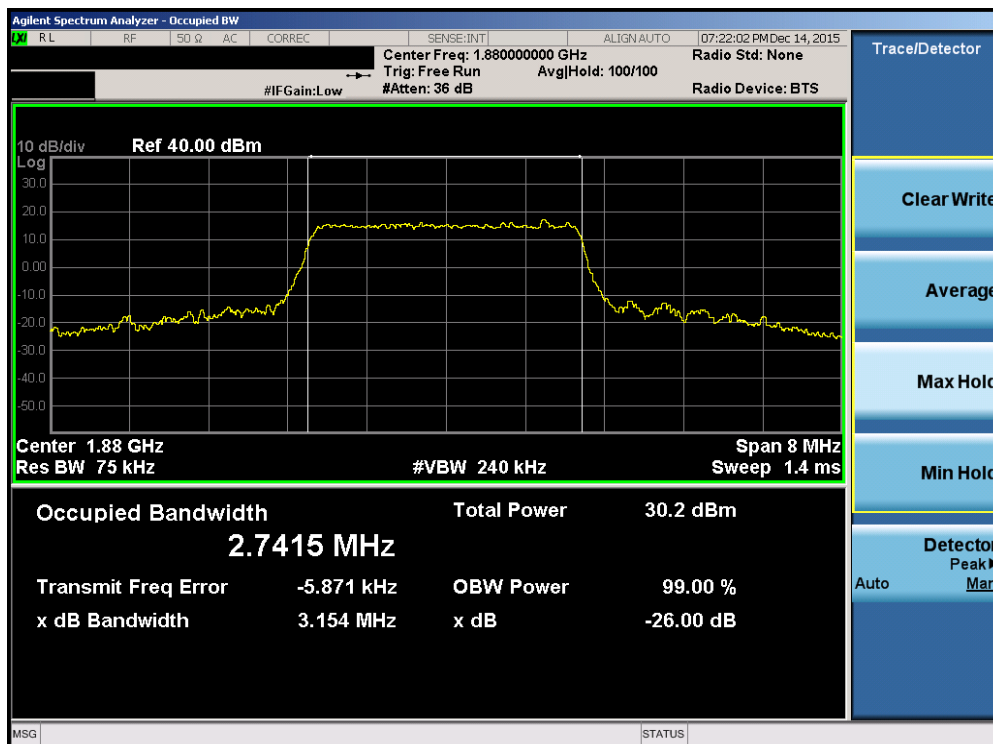
Plot 7-32. Occupied Bandwidth Plot (Band 2 – 3.0MHz 16-QAM – RB Size 15)
