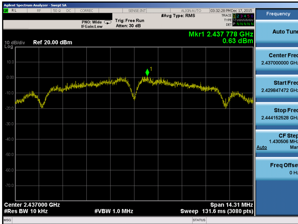
Plot 7-11. Power Spectral Density Plot (802.11b – Ch. 6)
