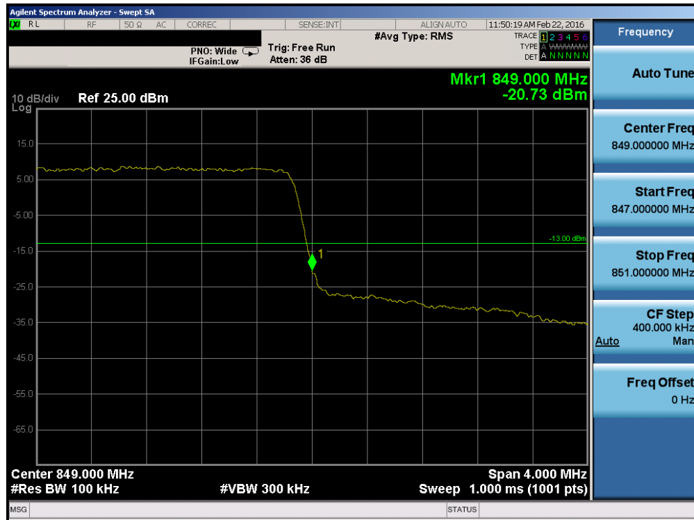
Plot 7-61. Upper Band Edge Plot (Band 26 – 3.0MHz QPSK – RB Size 15)
