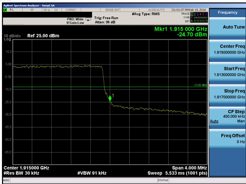
Plot 7-74. Upper Band Edge Plot (Band 25 – 3.0MHz QPSK – RB Size 15)
