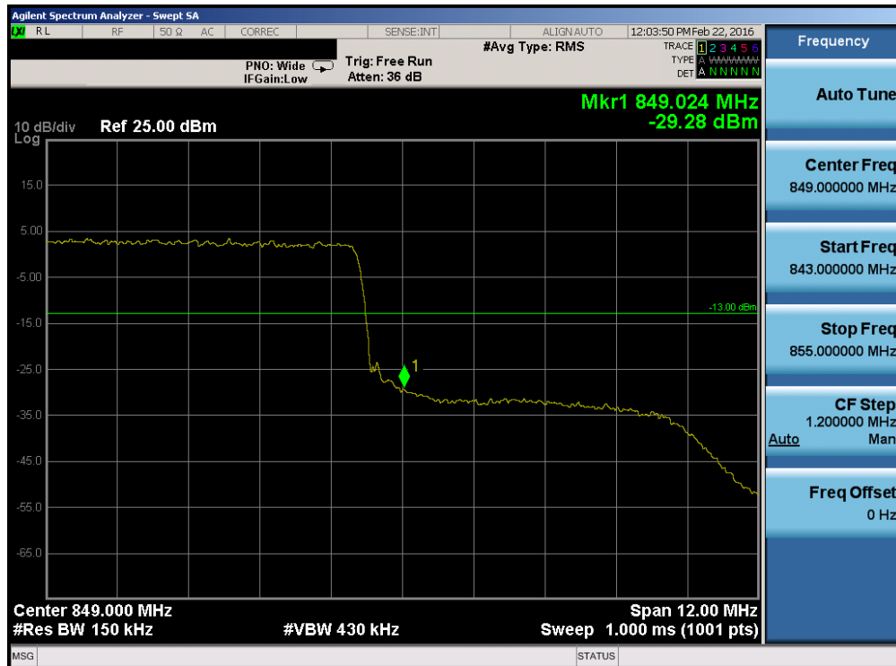
Plot 7-67. Upper Band Edge Plot (Band 26 – 15.0MHz QPSK – RB Size 75)
