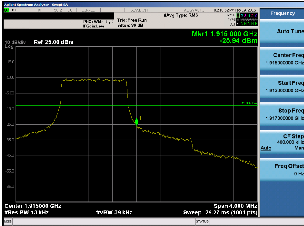
Plot 7-70. Upper Band Edge Plot (Band 25 – 1.4MHz QPSK – RB Size 6)
