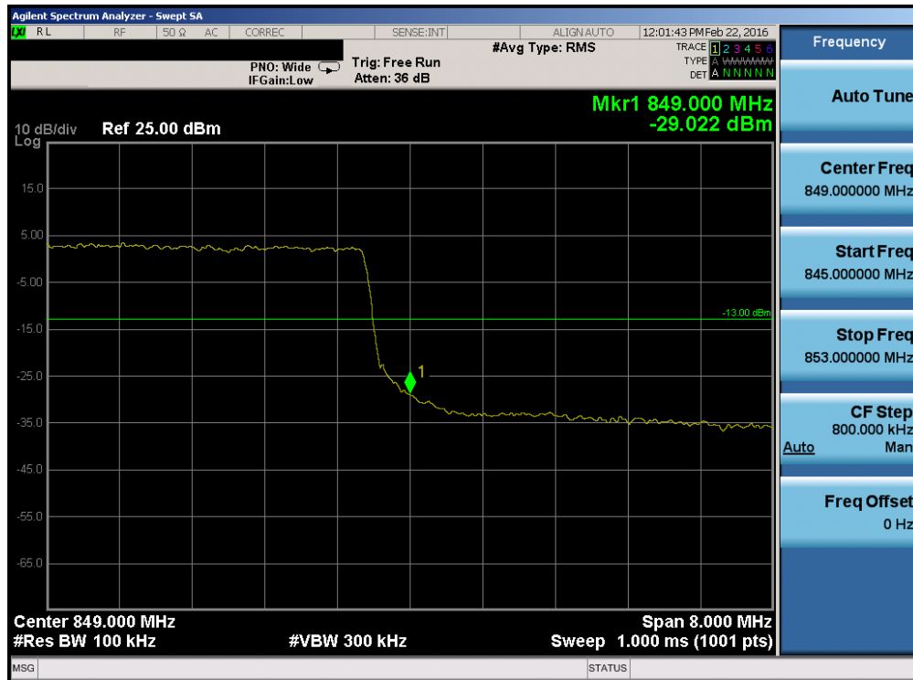
Plot 7-65. Upper Band Edge Plot (Band 26 – 10.0MHz QPSK – RB Size 50)
