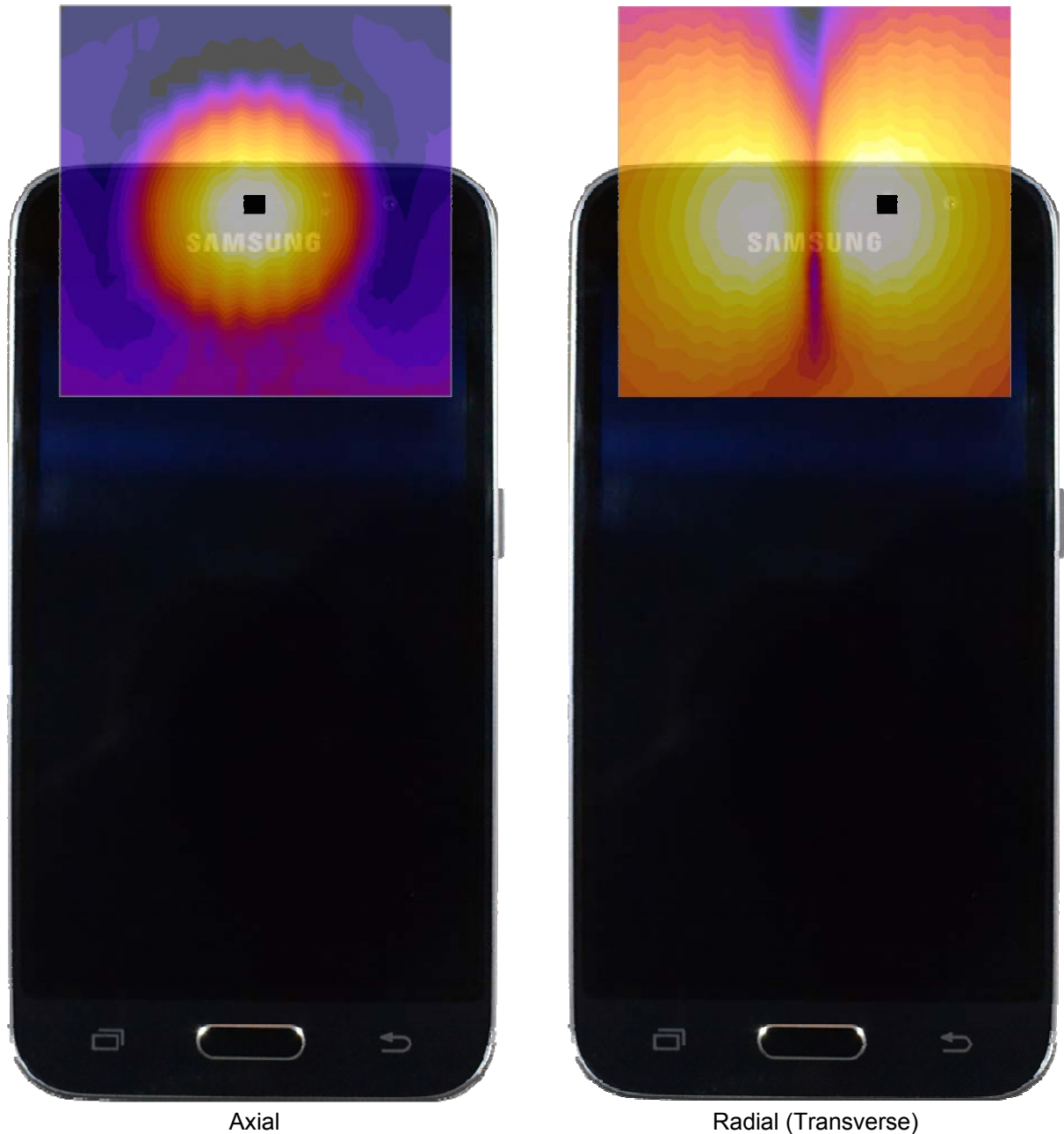
Figure 14-3 T-Coil Scan Overlay Magnetic Field Distributions
