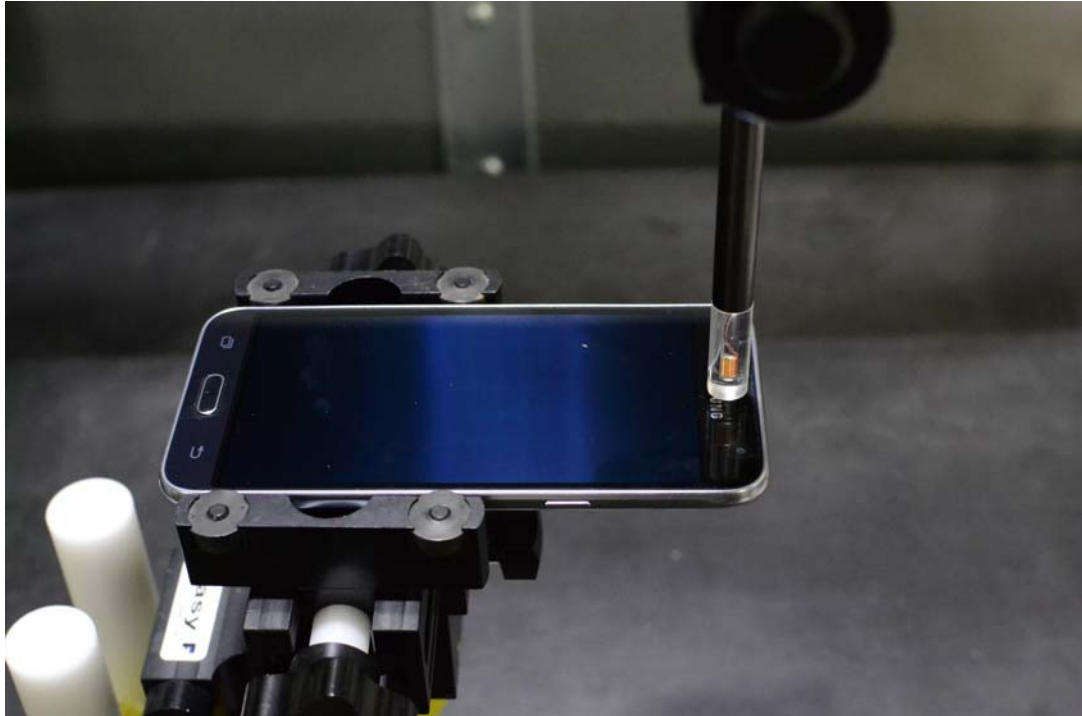
Figure 14-1 Test Setup for Wireless Device
