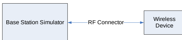
Figure 9-1 Power Measurement Setup
