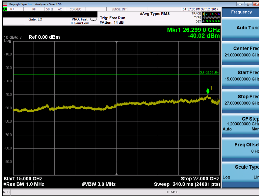
Plot 7-29. Conducted Spurious Plot (Band 38 – 10.0MHz QPSK – RB Size 1, RB Offset 0 – Low Channel)
