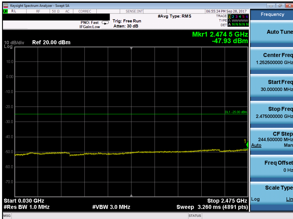
Plot 7-18. Conducted Spurious Plot (Band 7 - 10.0MHz QPSK - RB Size 1, RB Offset 0 - Low Channel)
