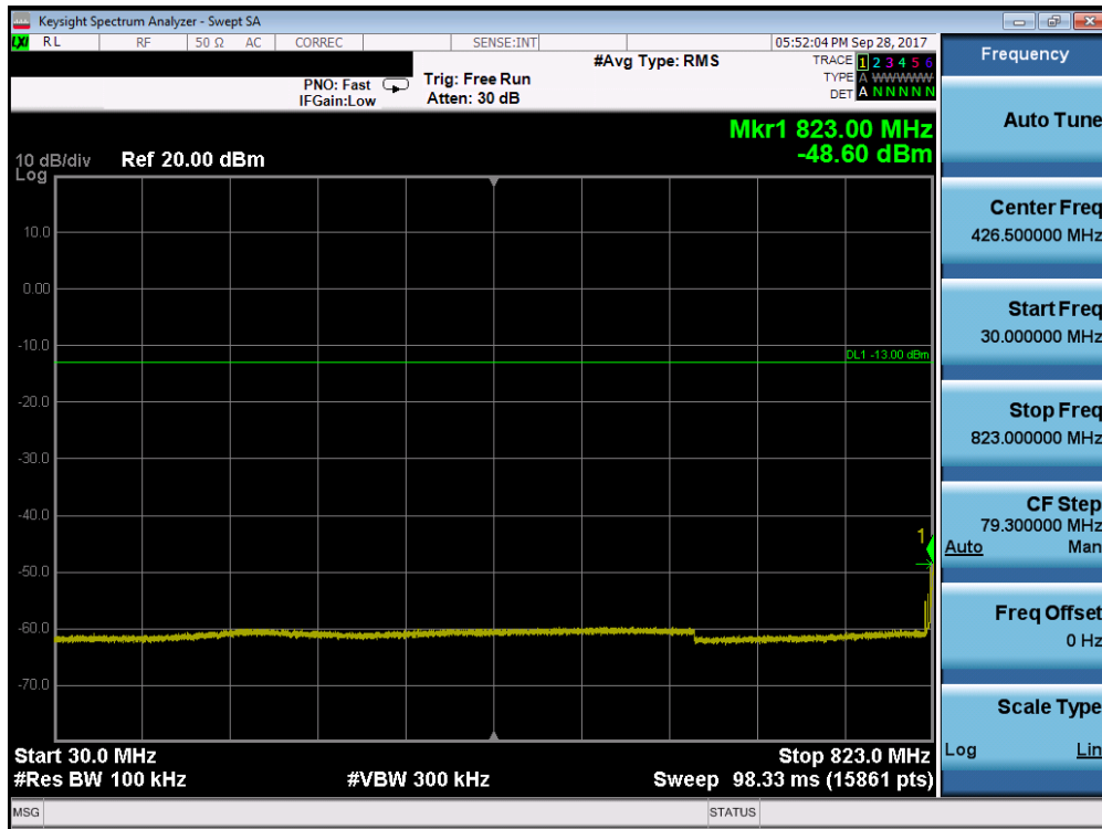
Plot 7-9. Conducted Spurious Plot (Band 5 - 10.0MHz QPSK - RB Size 1, RB Offset 0 - Low Channel)
