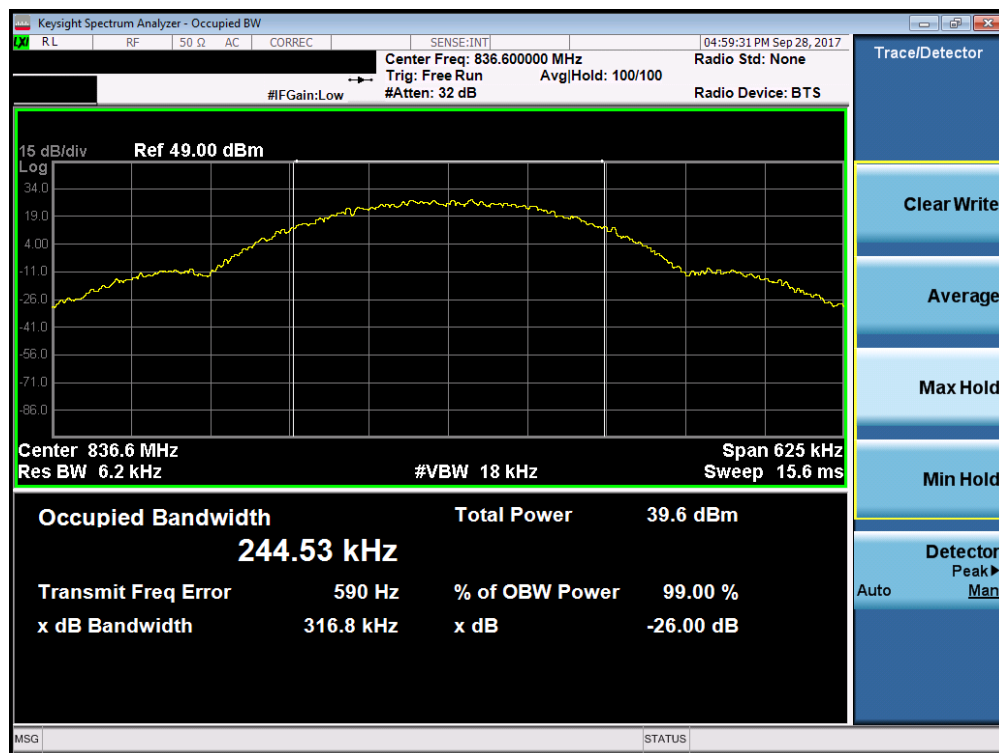
Plot 7-1. Occupied Bandwidth Plot (Cellular GPRS Mode)
