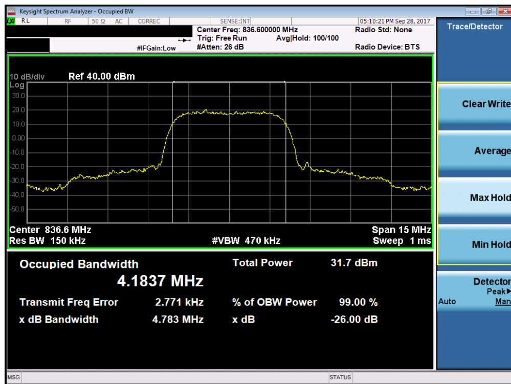
Plot 7-3. Occupied Bandwidth Plot (Cellular WCDMA Mode)
