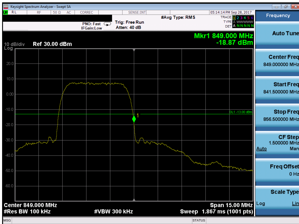
Plot 7-25. Band Edge Plot (Cellular WCDMA Mode - High Channel)
