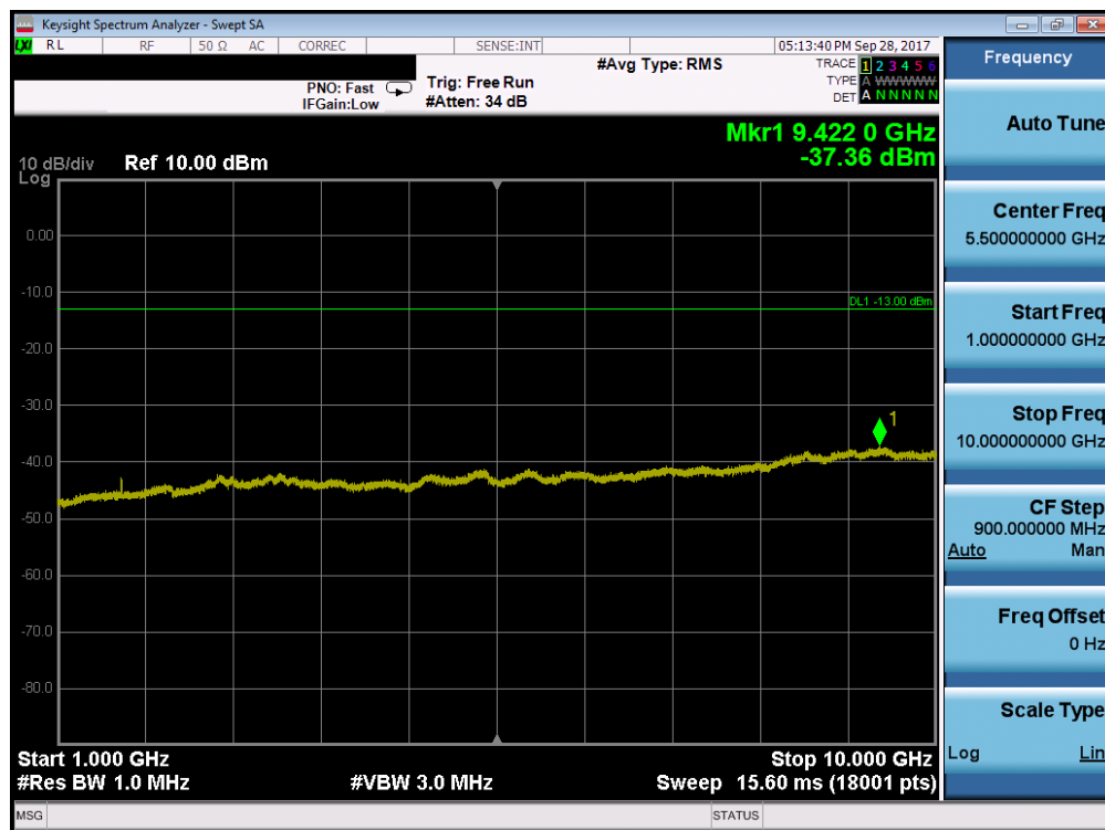
Plot 7-15. Conducted Spurious Plot (Cellular WCDMA Mode - Low Channel)
