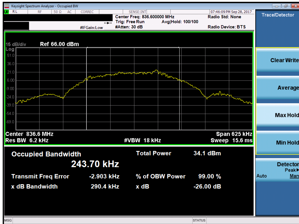
Plot 7-2. Occupied Bandwidth Plot (EDGE850 Mode)
