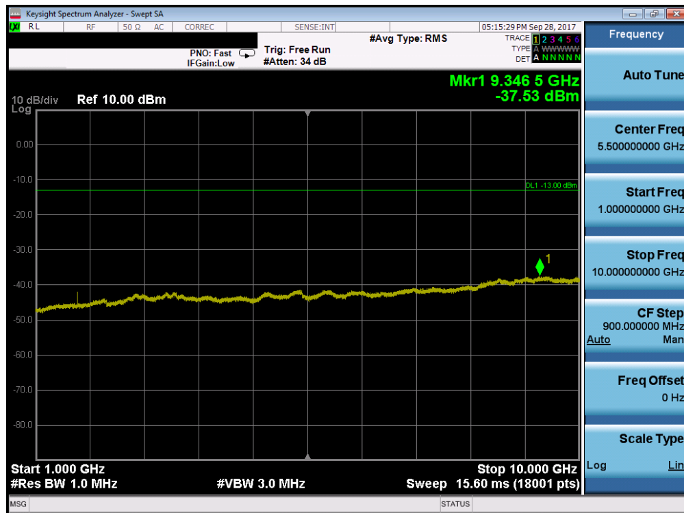
Plot 7-21. Conducted Spurious Plot (Cellular WCDMA Mode - High Channel)
