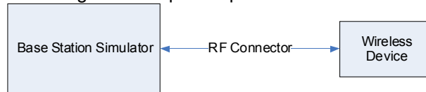
Figure 9-2 Power Measurement Setup
