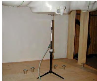
Figure 10-2 System Verification Setup Photo
