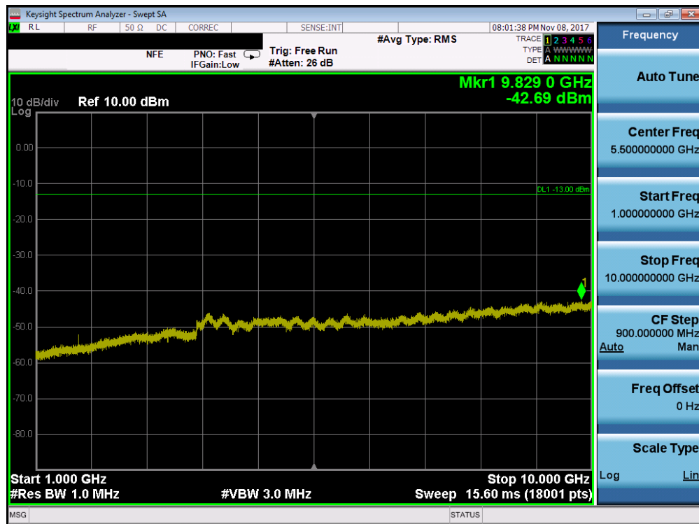
Plot 7-34. Conducted Spurious Plot (Cellular WCDMA Mode - High Channel)
