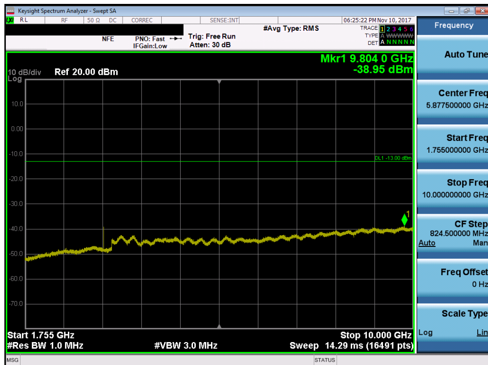
Plot 7-36. Conducted Spurious Plot (AWS WCDMA Mode - Low Channel)
