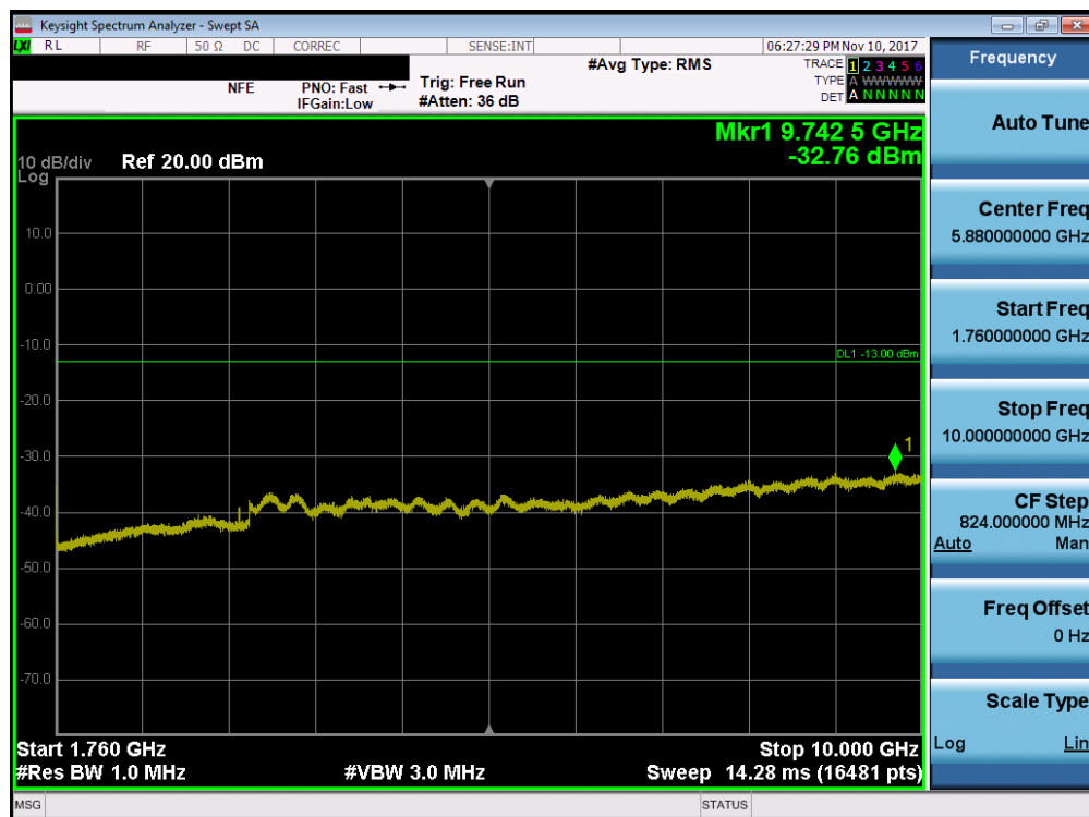
Plot 7-42. Conducted Spurious Plot (AWS WCDMA Mode - High Channel)
