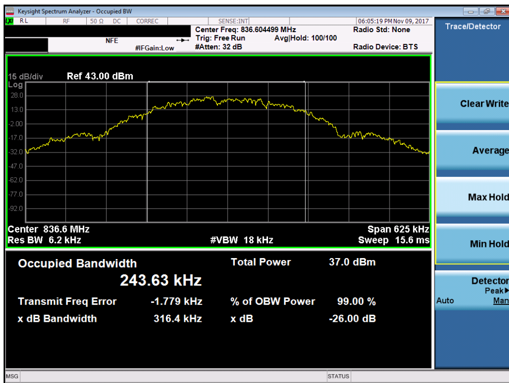
Plot 7-1. Occupied Bandwidth Plot (Cellular GSM Mode)
