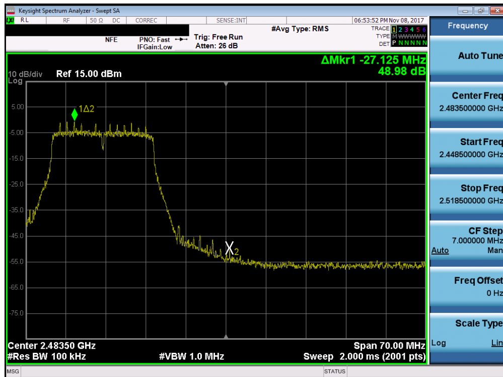
Plot 7-24. Band Edge Plot (802.11n (2.4GHz) – Ch. 11)
