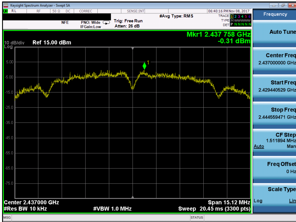
Plot 7-11. Power Spectral Density Plot (802.11b – Ch. 6)
