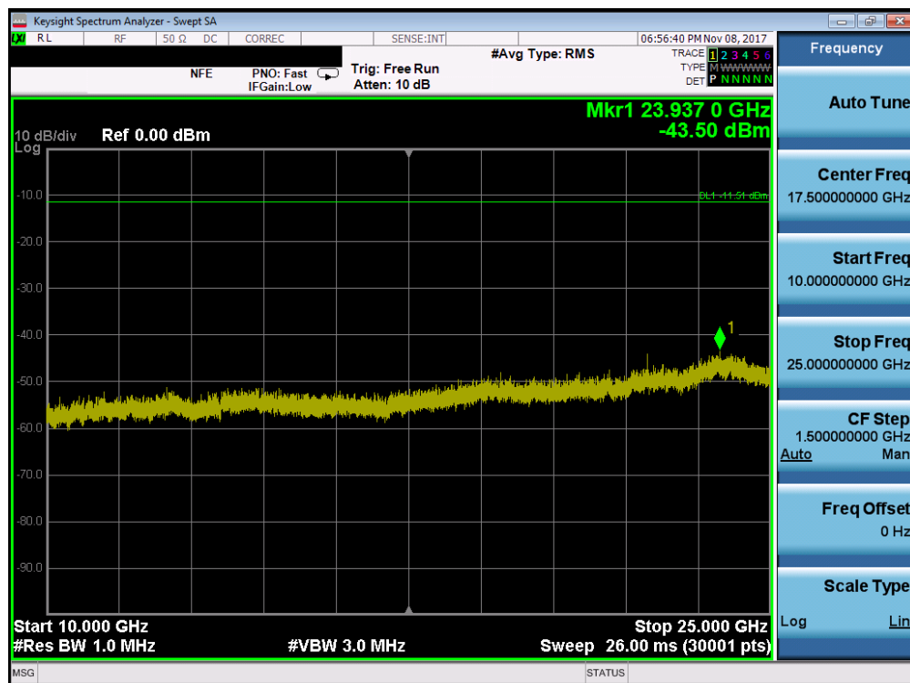
Plot 7-28. Conducted Spurious Plot (802.11b – Ch. 6)
