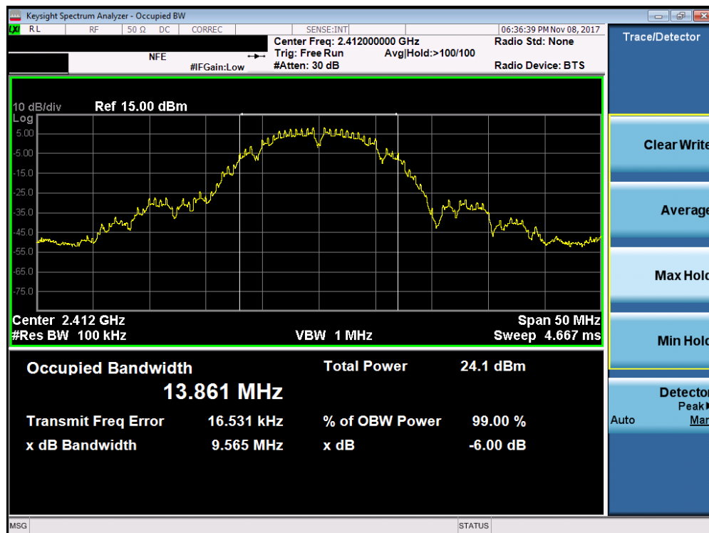
Plot 7-1. 6dB Bandwidth Plot (802.11b – Ch. 1)
