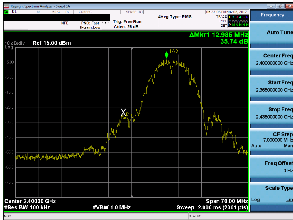
Plot 7-19. Band Edge Plot (802.11b – Ch. 1)
