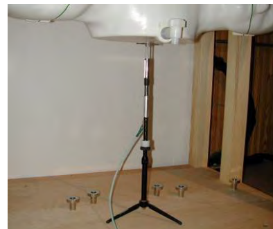
Figure 10-2 System Verification Setup Photo
