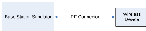
Figure 9-2 Power Measurement Setup
