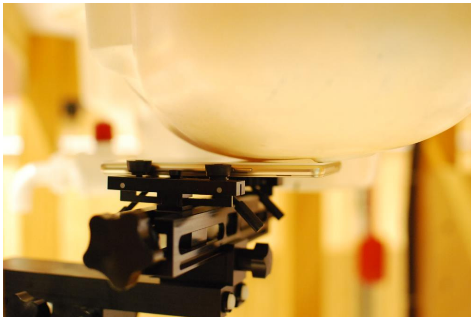
SAR Test Setup Photo 3 – Left Cheek
