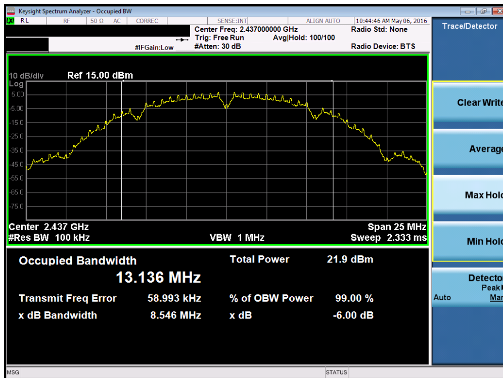
Plot 7-2. 6dB Bandwidth Plot (802.11b – Ch. 6)
